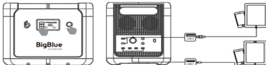
1. Turn on the power switch (press and hold for 3 seconds), the screen will light up. Click the DC icon on the screen to turn on the DC, USB-A, USB-C output.
