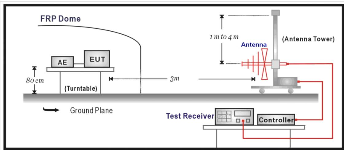
1GHz -40GHz Test Setup:
