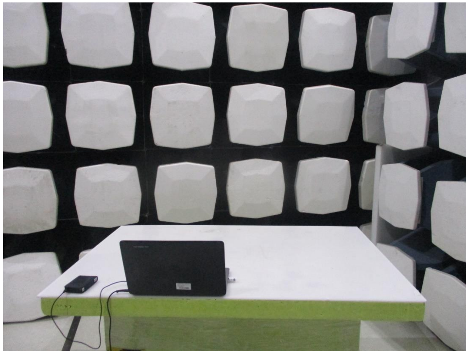
The EUT is placed at the center of turntable
