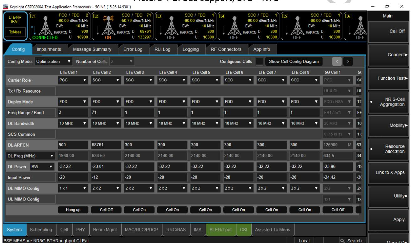
Picture 4-3: DSS support, B71 + N71, downlink 135 Mbps. Can be stable transmission without NACK.
