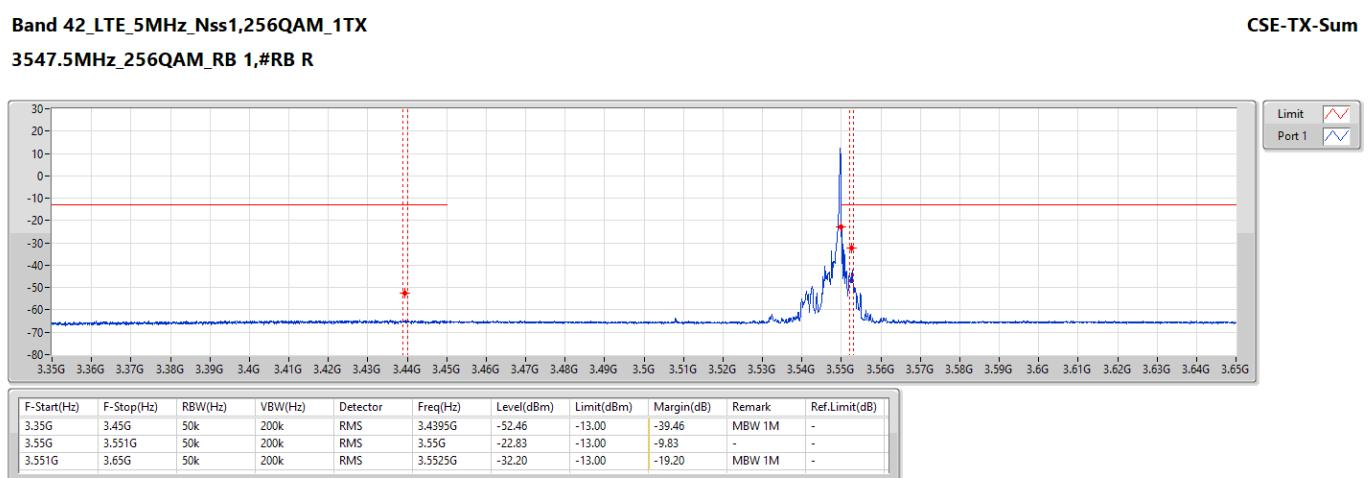
Note 1: Measured level is integrated to 1 MHz bandwidth by lower RBW setting and band power measurement function for remark item.
