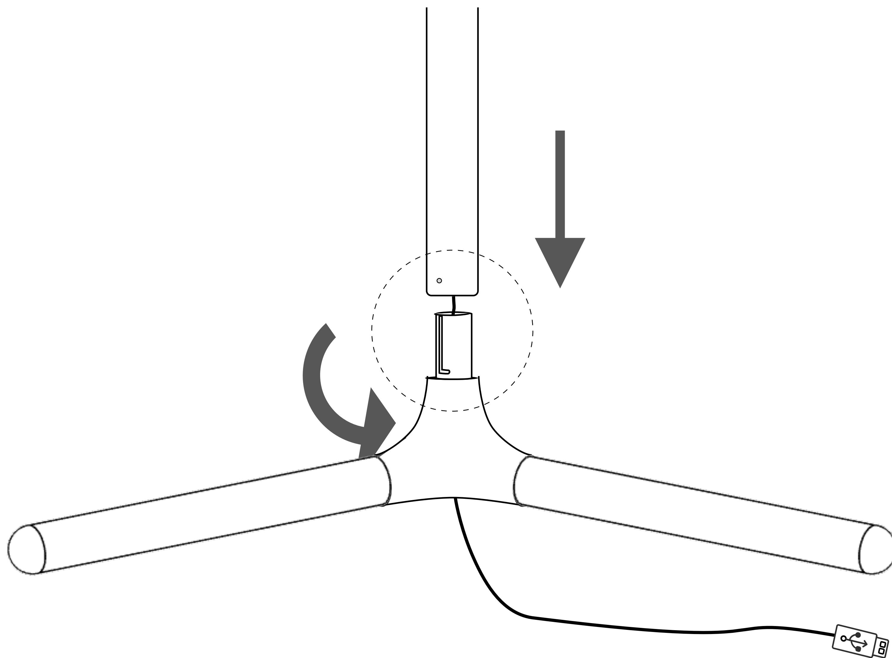
Push the USB cord through the rest of the EXTENSION TUBE in sequence, and mount them together by screwing the EXTENSION TUBE. Choose between three EXTENSION TUBEs or two EXTENSION TUBEs as instructed.
