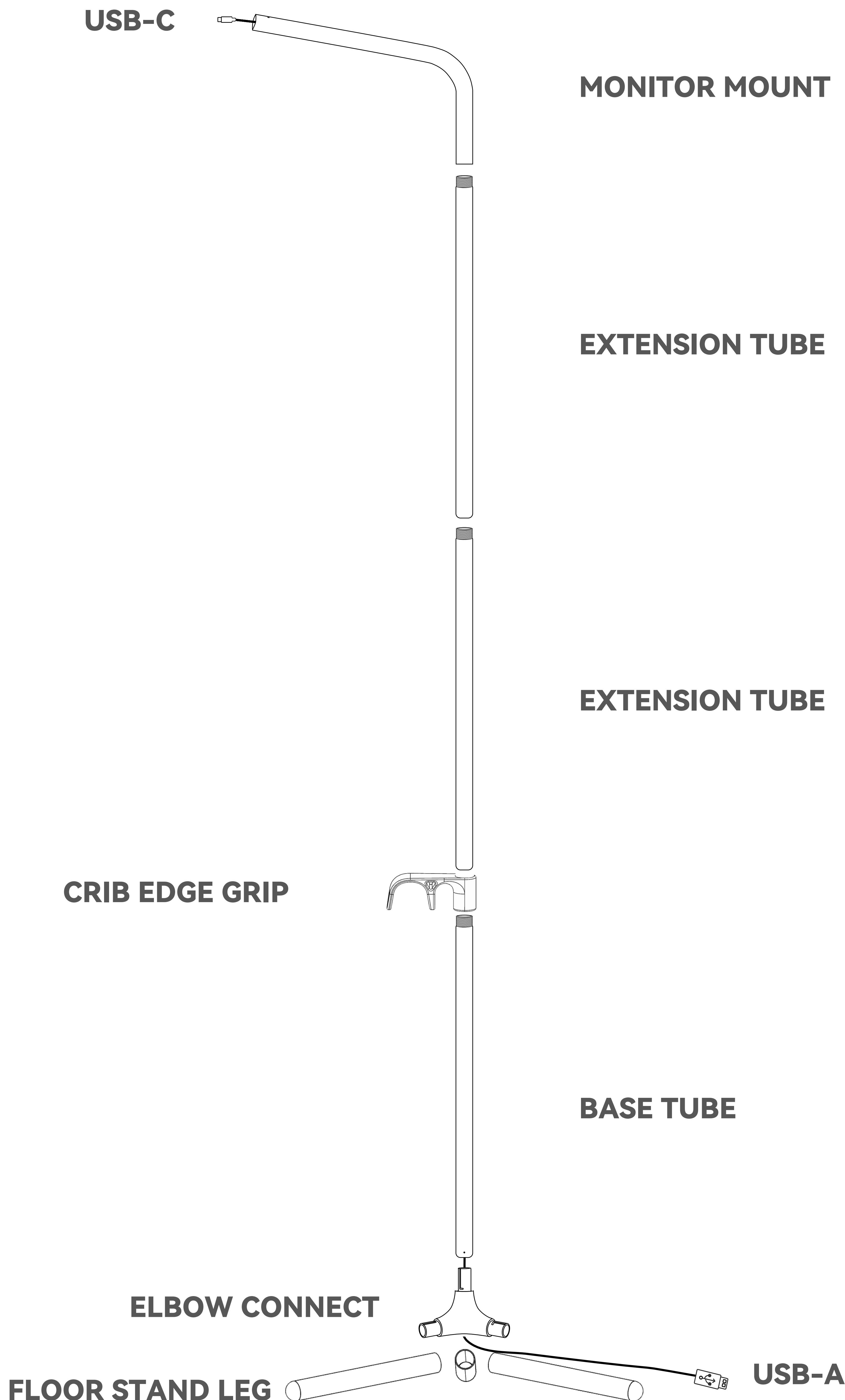
Screw three FLOOR STAND LEGs and ELBOW CONNECT together.
