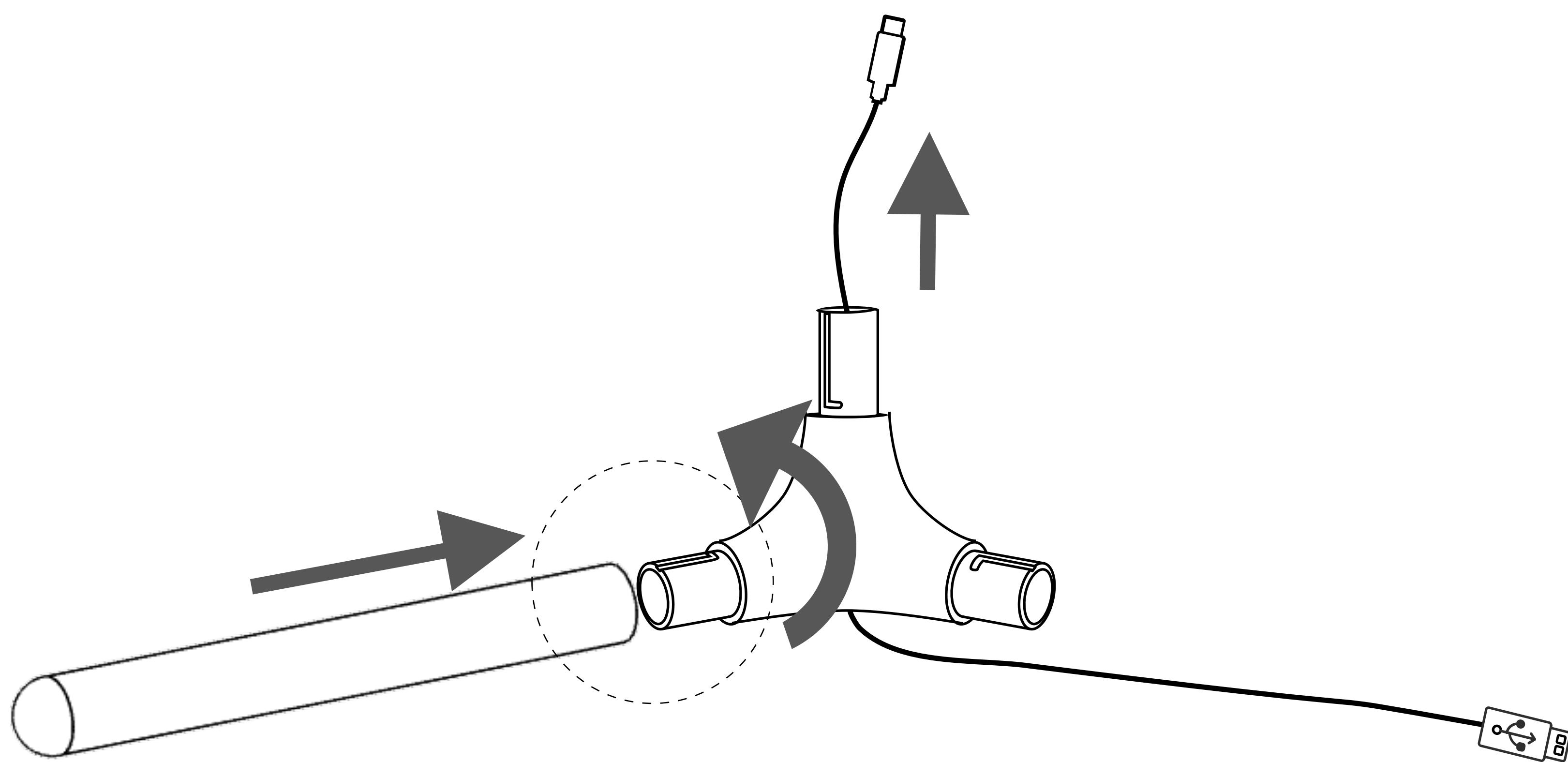
Push together the MOUNT to the BASE TUBE and second EXTENSION TUBE and RETRACTABLE TUBE. Then screw RETRACTABLE TUBE and ELBOW CONNECT together.
