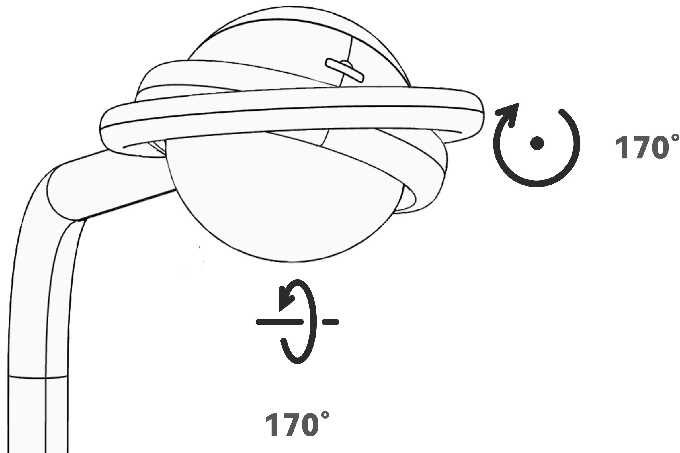
Rotate AXIS HALO to reveal the position of the TF card slot, remove the TF card slot cover, insert side B vertically upward into the TF card slot until the TF card is locked, and then restore the TF card slot cover to its original position. Do not power off the device when operating the TF card.
