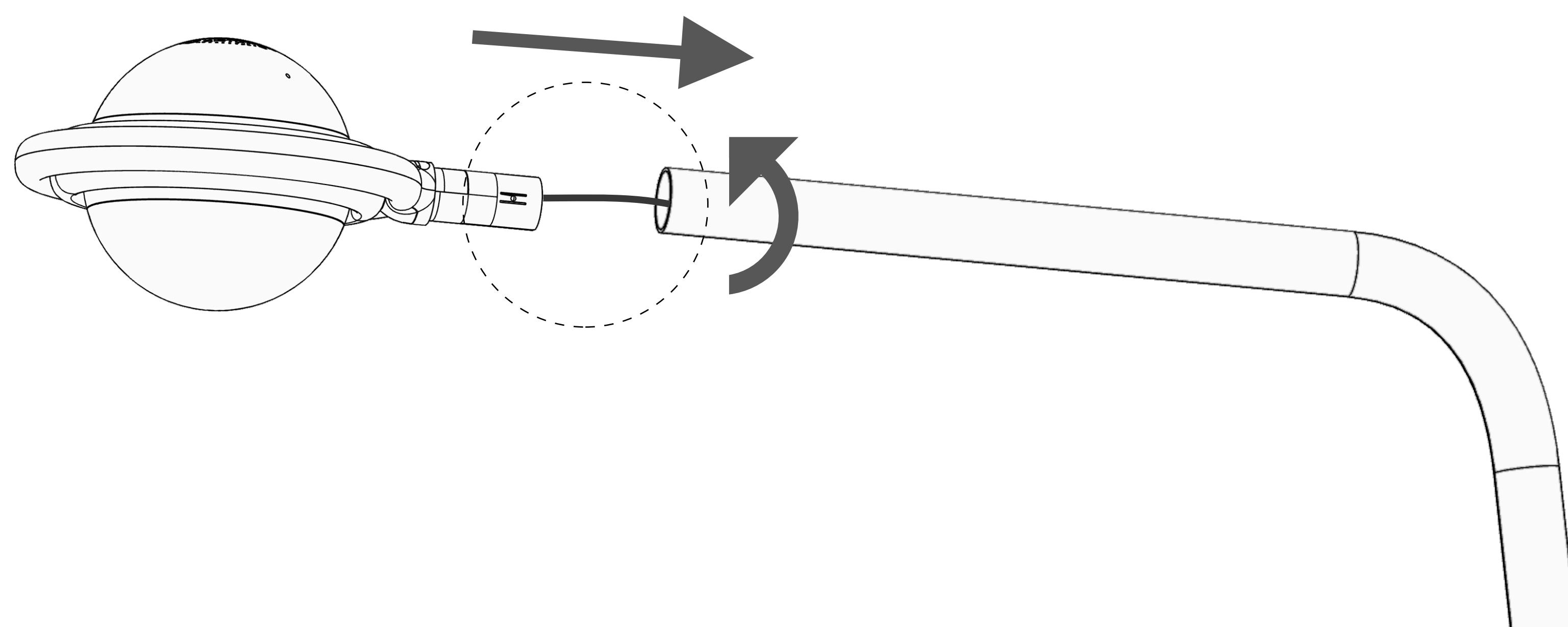
The MONITOR installed on the MOUNT can be manually rotated 170 degrees from front to back and 170 degrees from left to right to position its orientation. The appropriate Angle needs to be adjusted according to the live stream screen in the VitaRadar APP. Please refer to the application introduction of the APP for specific methods.
