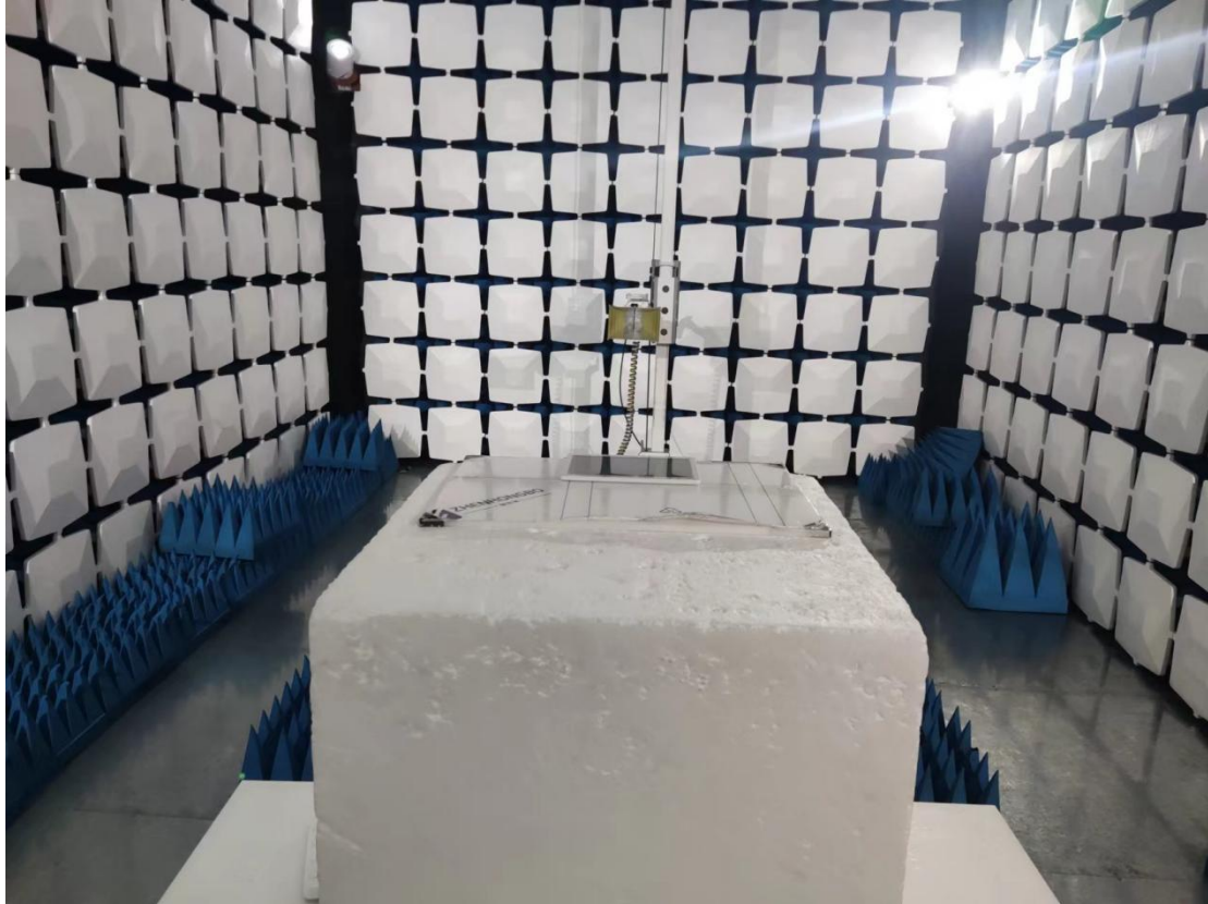
Above 1GHz for radiated emission test setup
