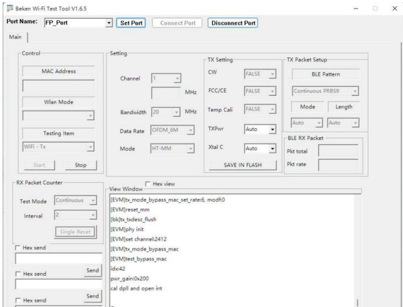
The test software was used to control EUT work in continuous TX mode, and select test channel, Wireless mode as below table
