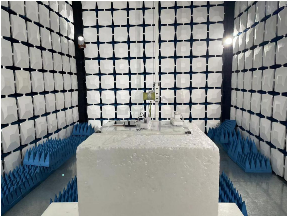
Above 1GHz for radiated emission test setup
