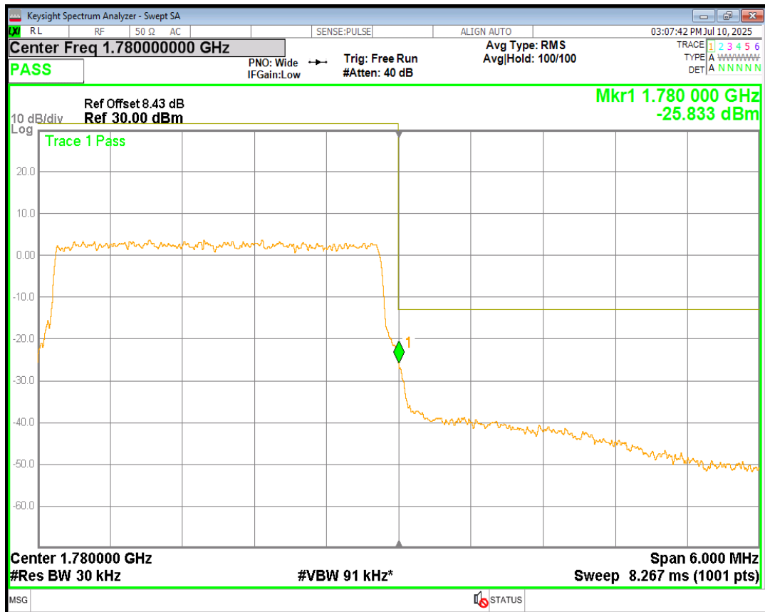
Band66 16QAM BW=5MHz Channel=131997 RB Size=25 Position=#0
