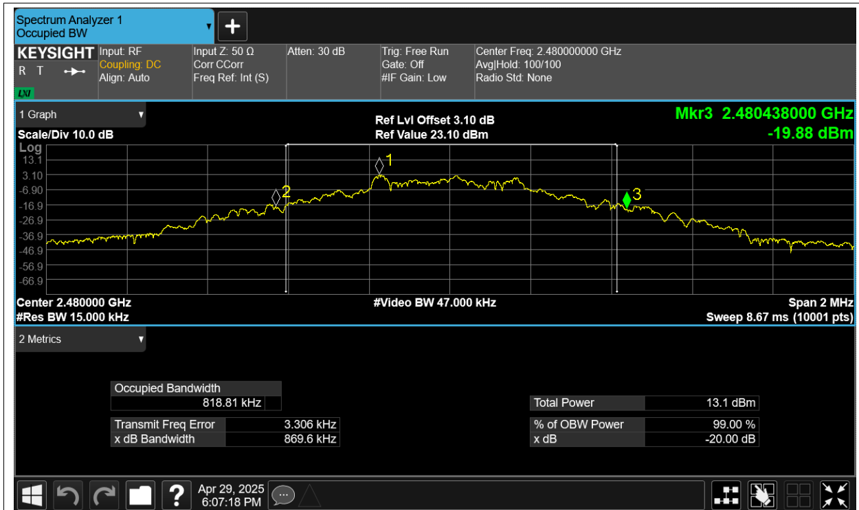
-20dB Bandwidth NVNT 2-DH1 2402MHz Ant1
