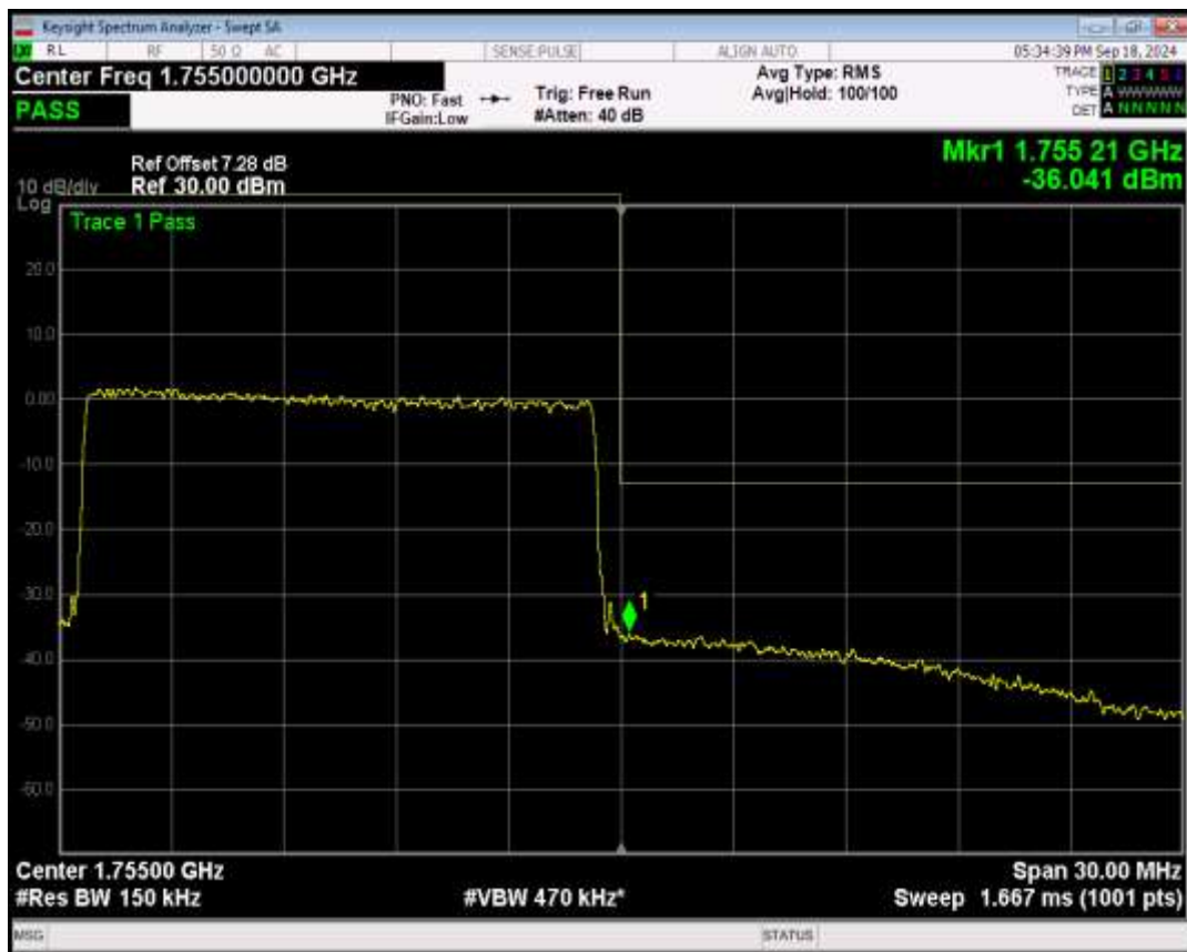
Band4 QPSK BW=20MHz Channel=20050 RB Size=1 Position=#0
