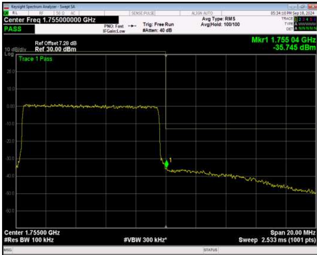
Band4 16QAM BW=10MHz Channel=20350 RB Size=1 Position=#Max
