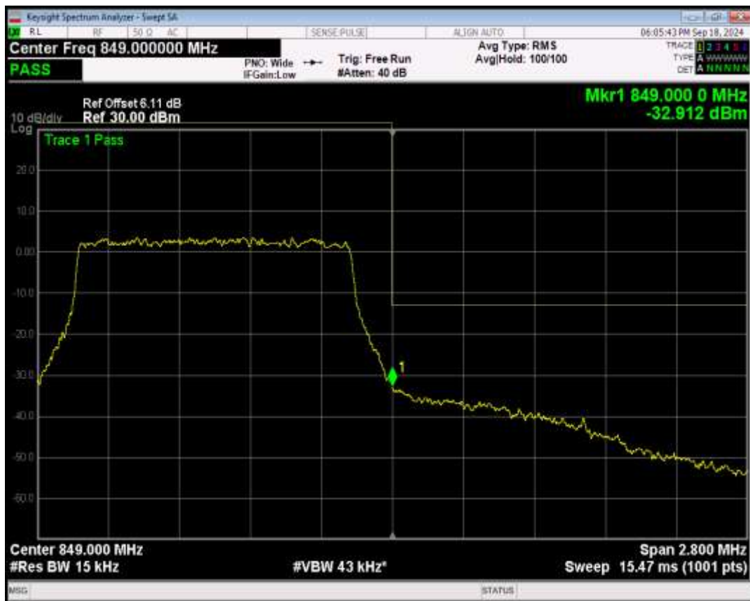
Band5 QPSK BW=3MHz Channel=20415 RB Size=1 Position=#0
