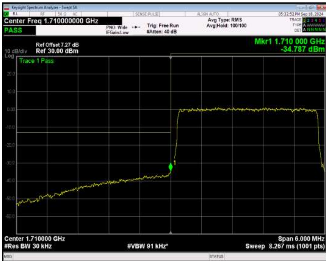
Band4 QPSK BW=3MHz Channel=20385 RB Size=1 Position=#0
