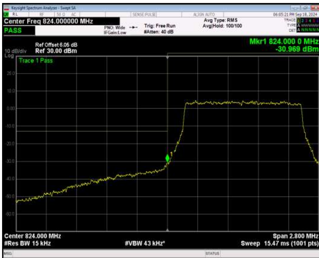
Band5 QPSK BW=1.4MHz Channel=20643 RB Size=1 Position=#Max
