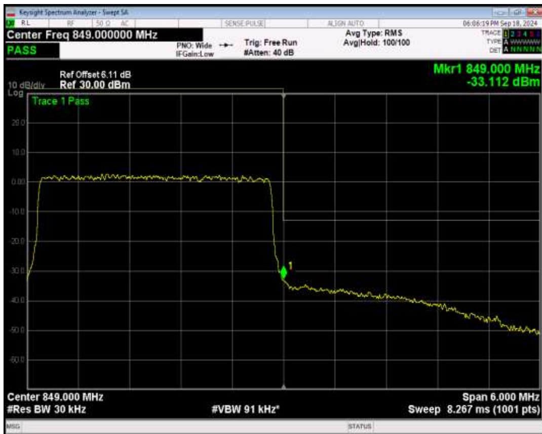
Band5 QPSK BW=5MHz Channel=20425 RB Size=1 Position=#0
