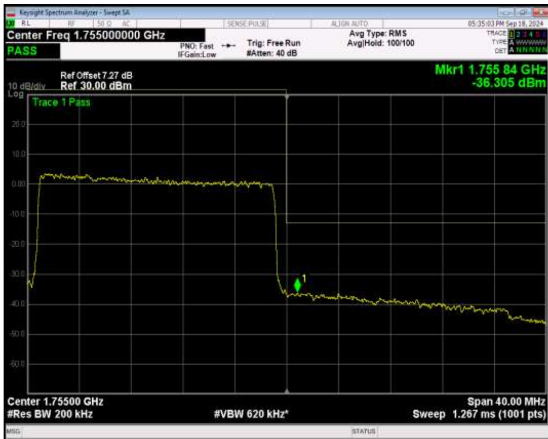
Band4 QPSK BW=20MHz Channel=20300 RB Size=1 Position=#Max
