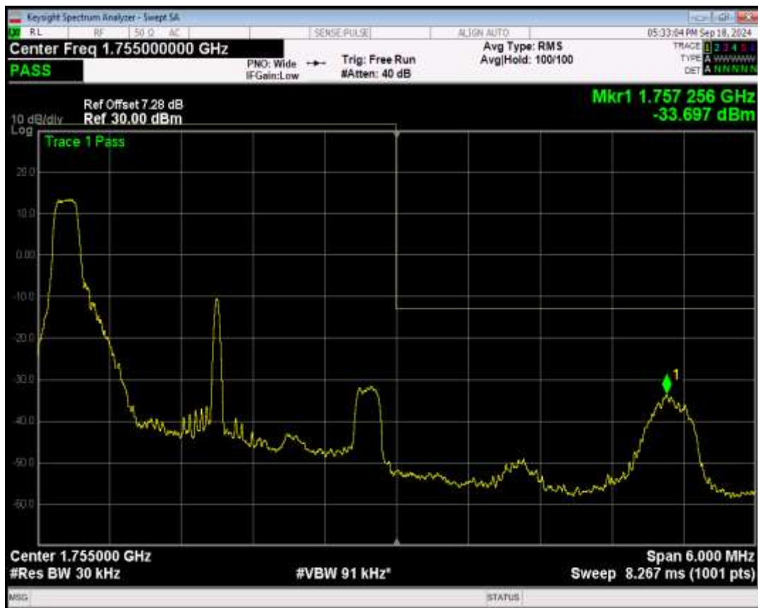
Band4 16QAM BW=3MHz Channel=20385 RB Size=1 Position=#Max
