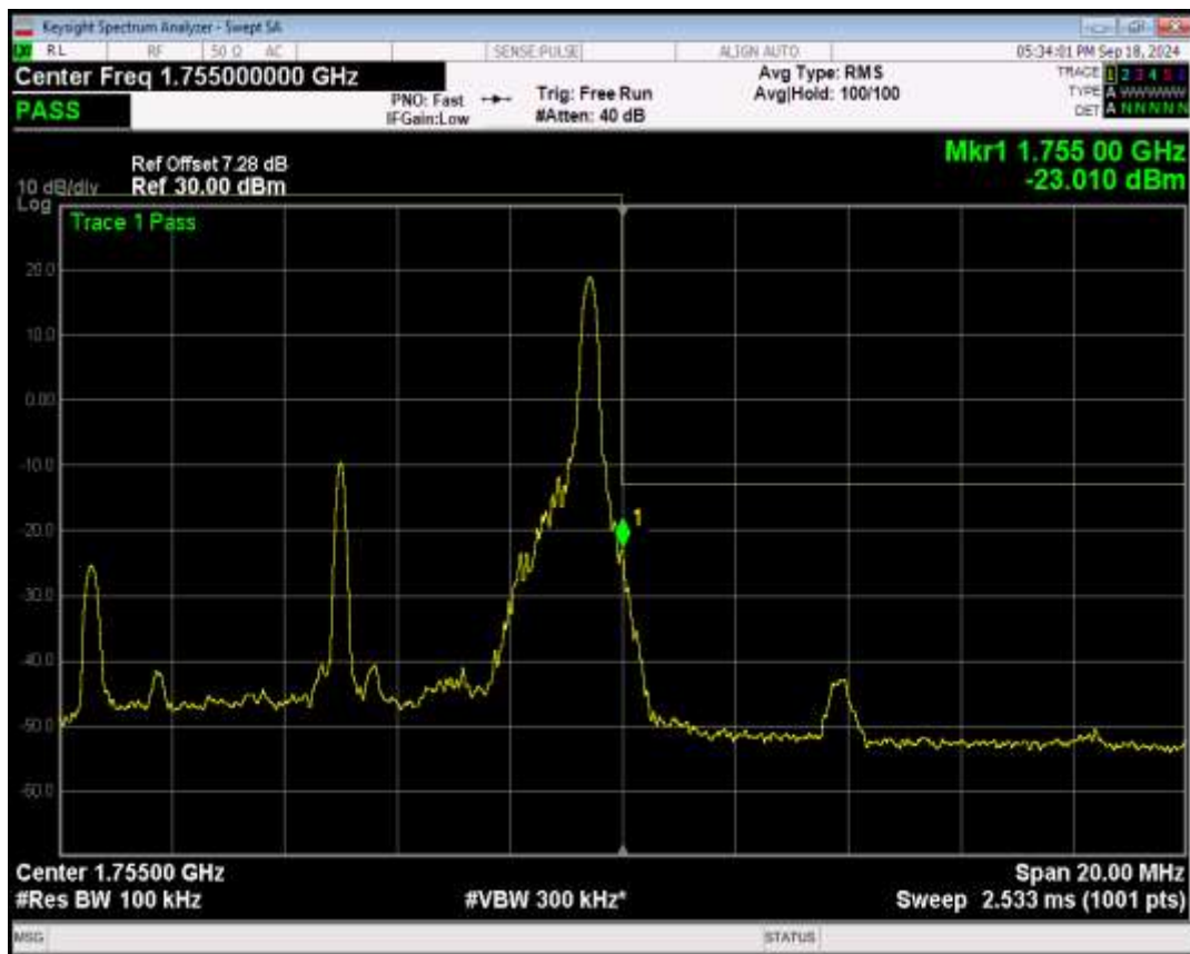
Band4 QPSK BW=10MHz Channel=20350 RB Size=50 Position=#0
