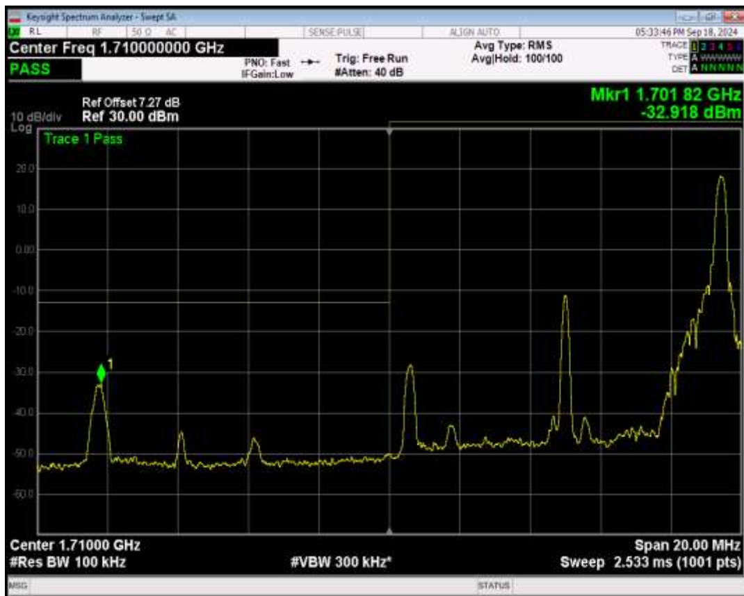
Band4 QPSK BW=10MHz Channel=20000 RB Size=50 Position=#0
