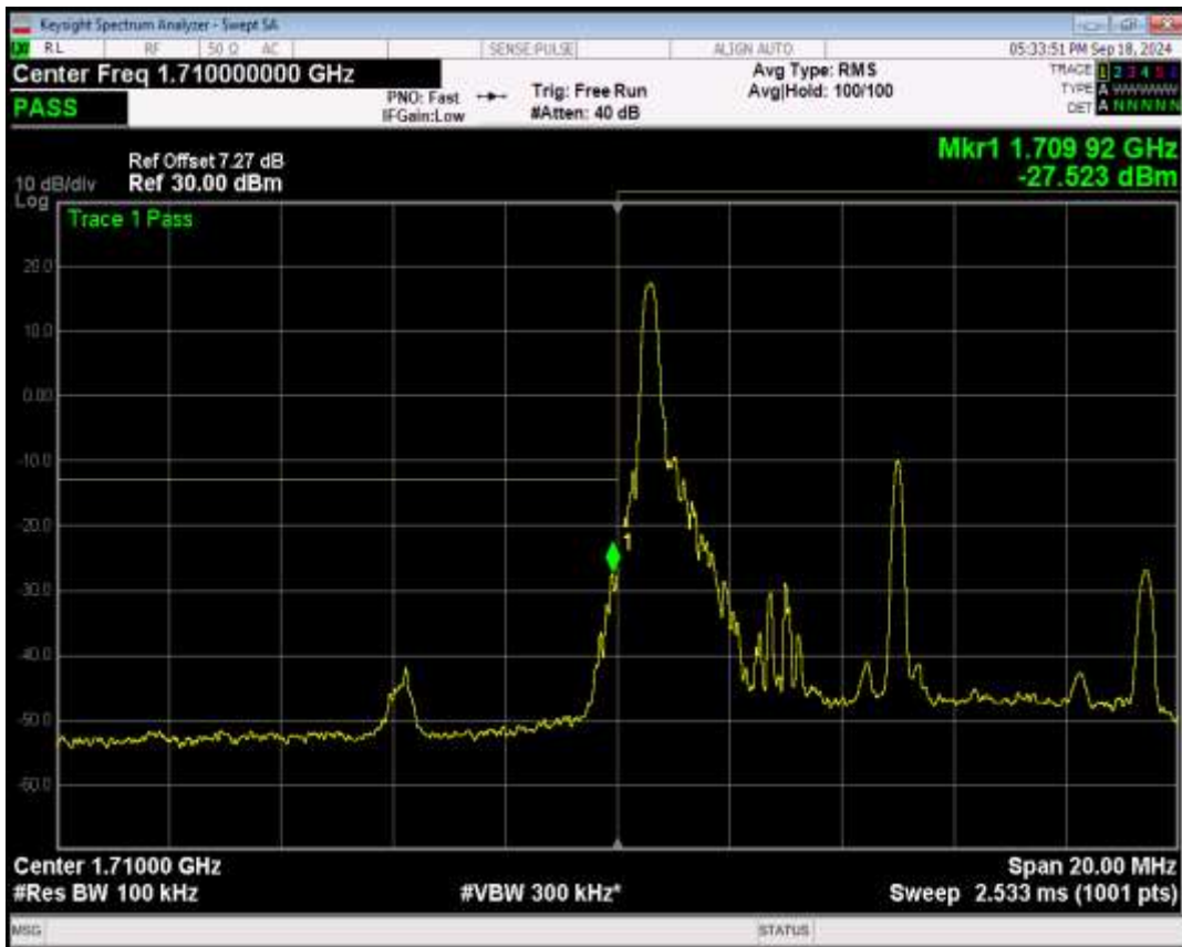
Band4 16QAM BW=10MHz Channel=20000 RB Size=1 Position=#Max
