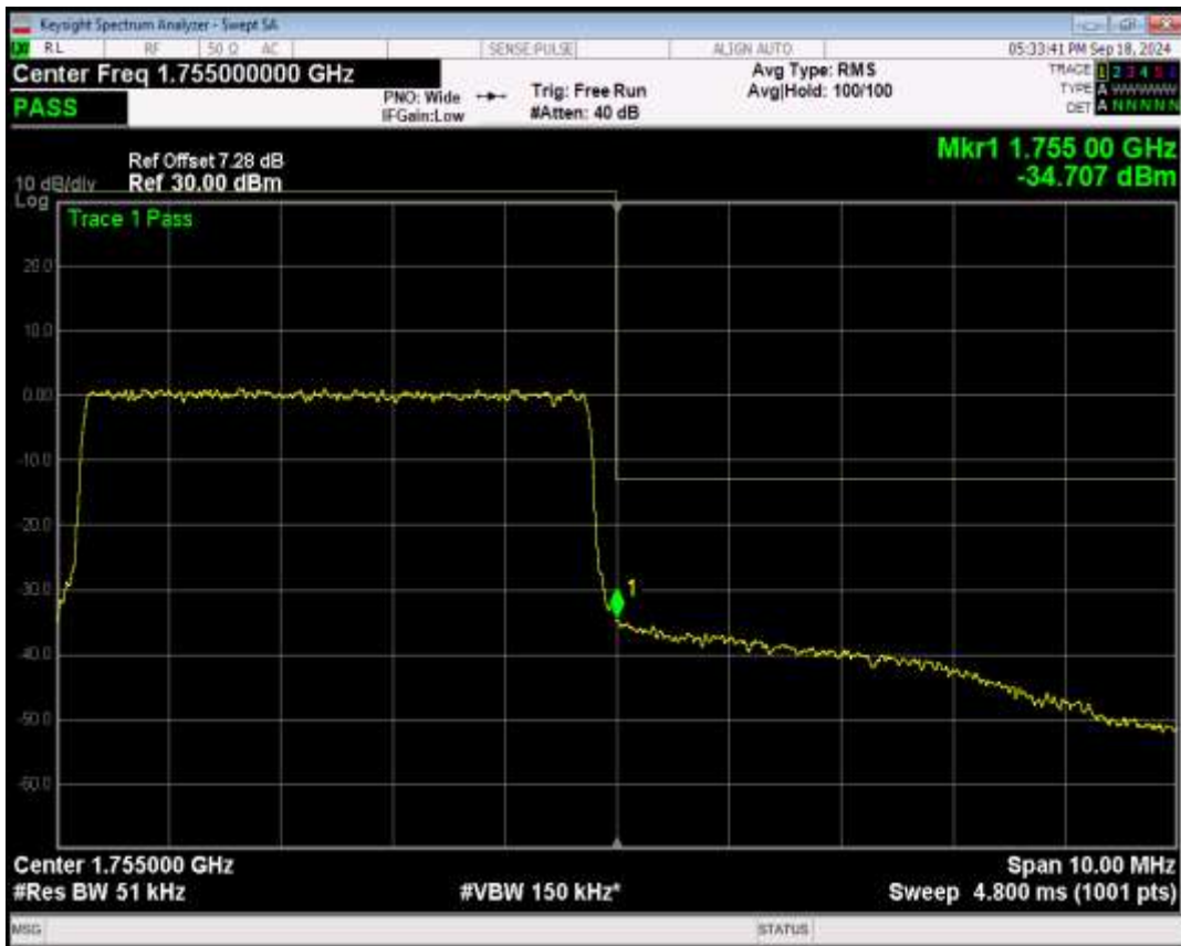
Band4 QPSK BW=10MHz Channel=20000 RB Size=1 Position=#0
