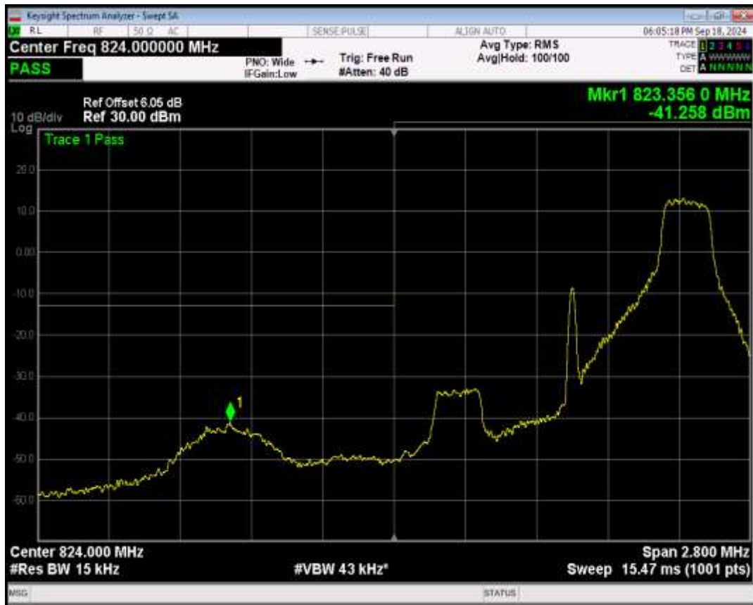
Band5 QPSK BW=1.4MHz Channel=20643 RB Size=1 Position=#0
