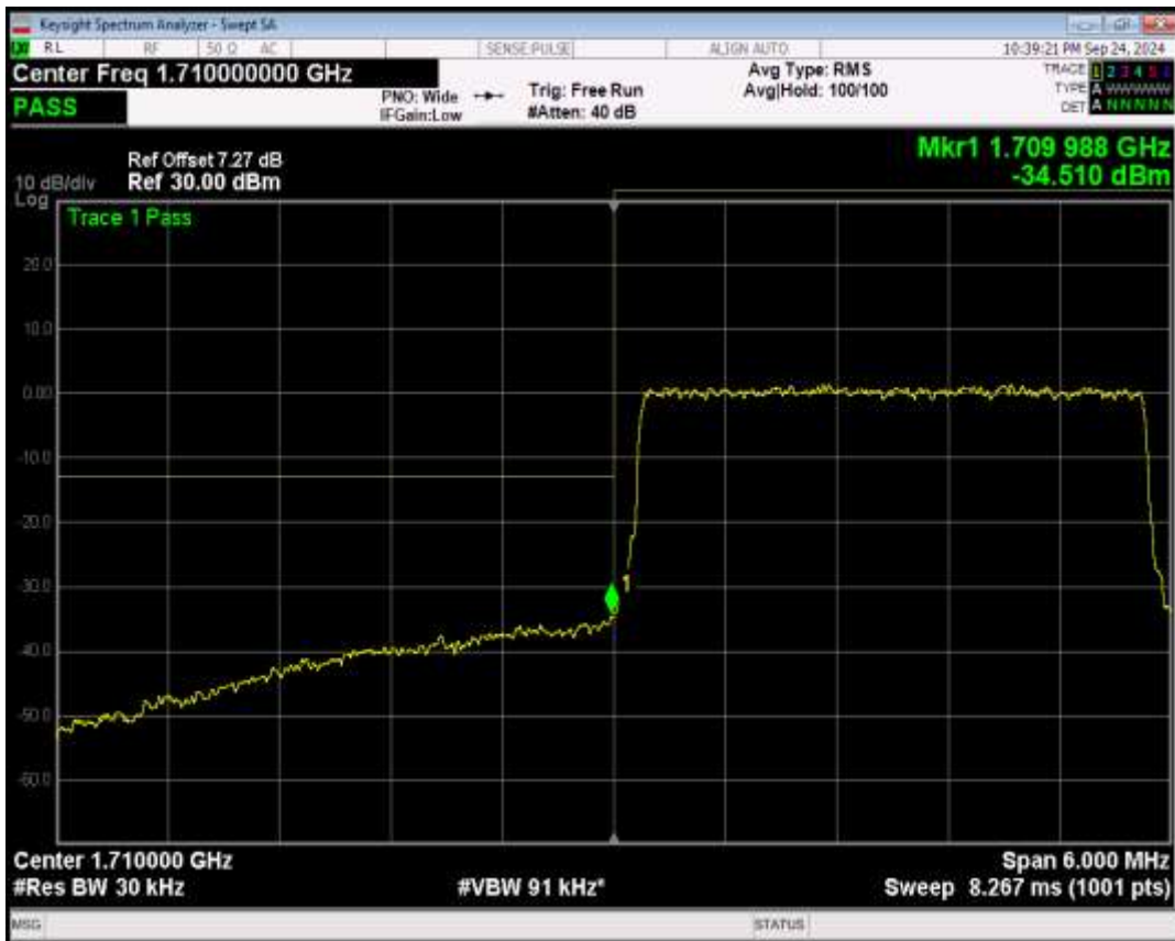
Band66 QPSK BW=3MHz Channel=132657 RB Size=1 Position=#0
