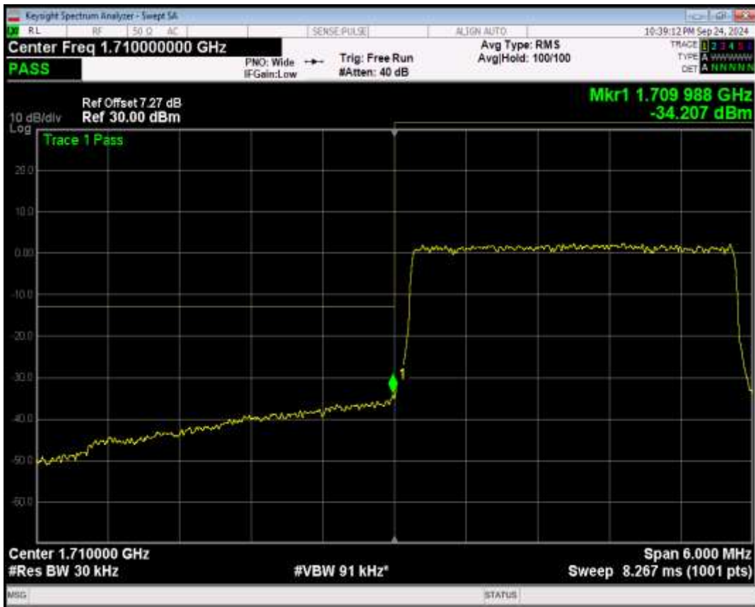
Band66 16QAM BW=3MHz Channel=131987 RB Size=1 Position=#0
