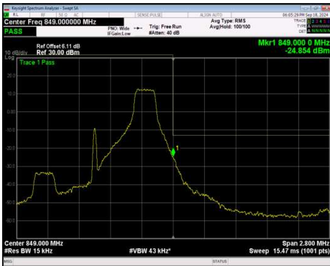
Band5 QPSK BW=1.4MHz Channel=20643 RB Size=6 Position=#0
