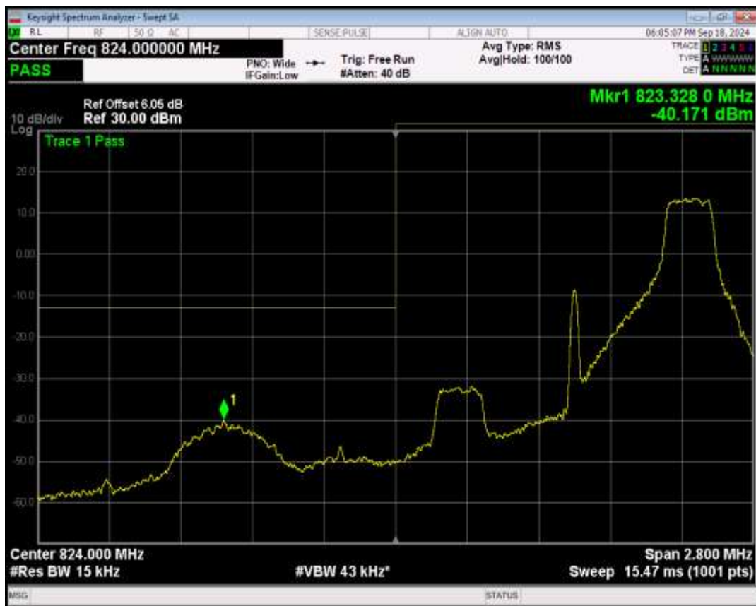
Band5 QPSK BW=1.4MHz Channel=20407 RB Size=6 Position=#0
