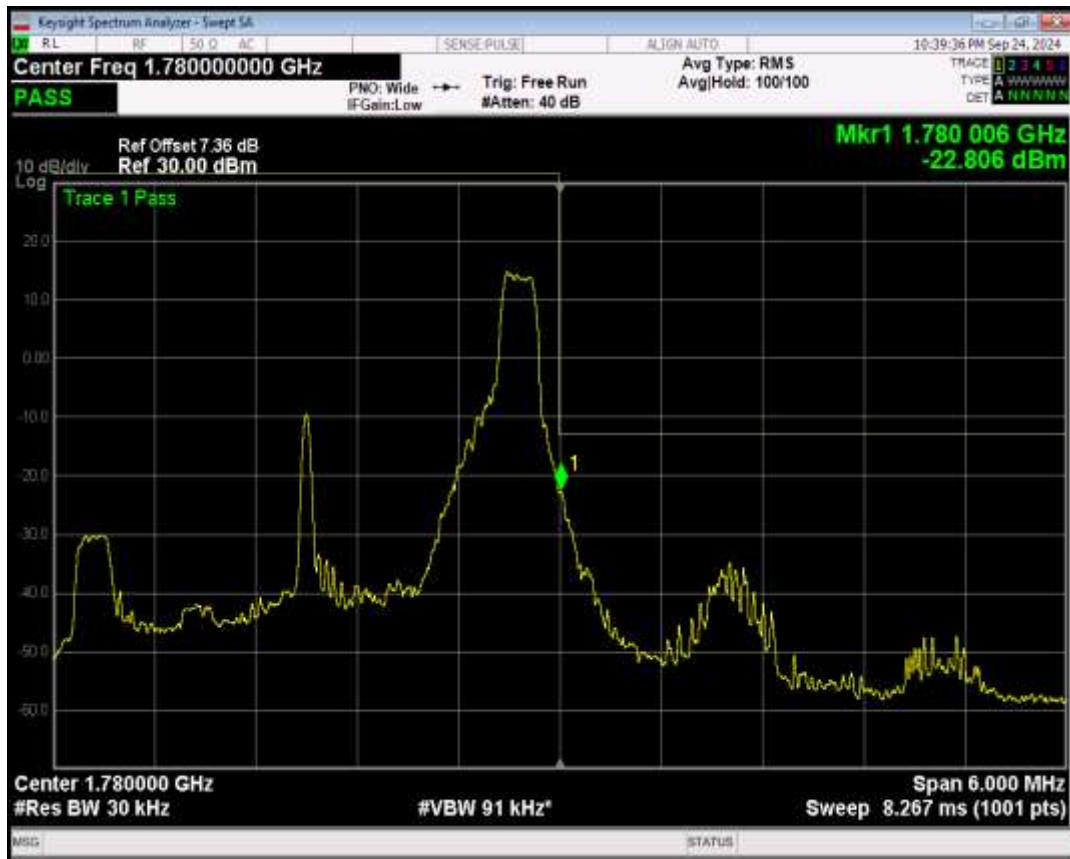
Band66 16QAM BW=3MHz Channel=132657 RB Size=15 Position=#0
