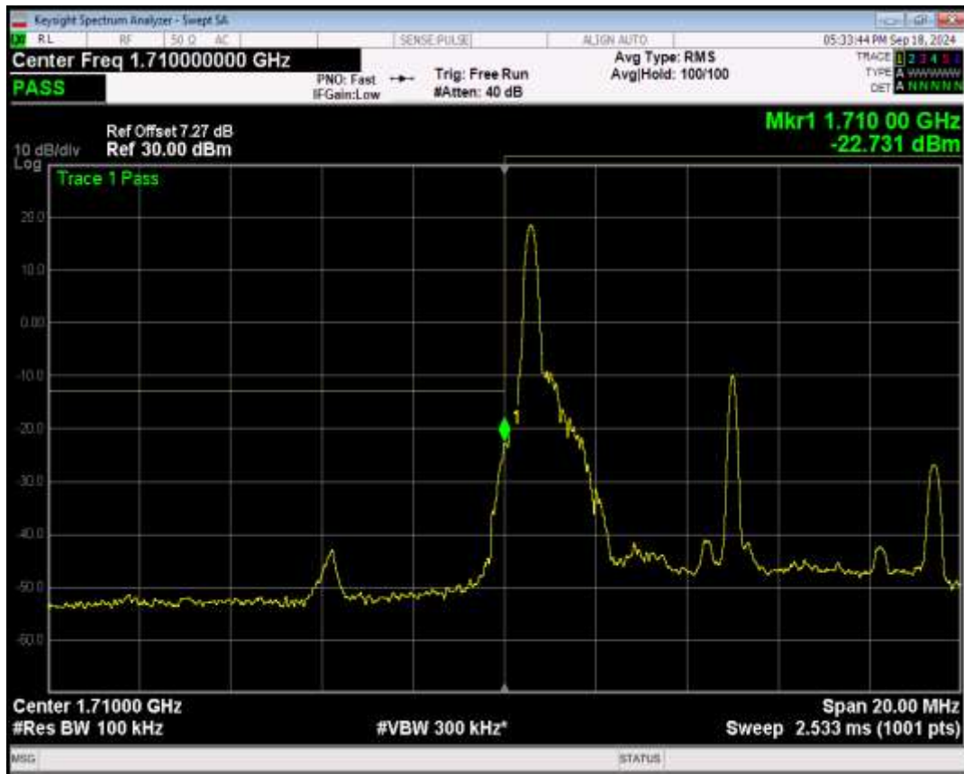
Band4 QPSK BW=10MHz Channel=20000 RB Size=1 Position=#Max
