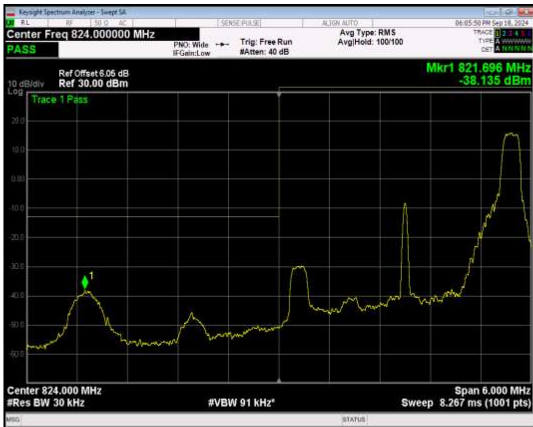
Band5 QPSK BW=3MHz Channel=20415 RB Size=15 Position=#0
