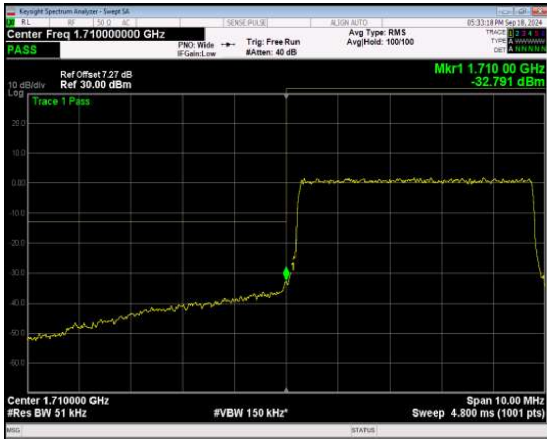
Band4 16QAM BW=5MHz Channel=19975 RB Size=1 Position=#0
