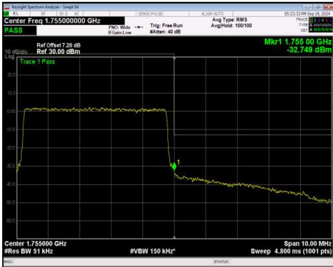
Band4 16QAM BW=5MHz Channel=20375 RB Size=1 Position=#0
