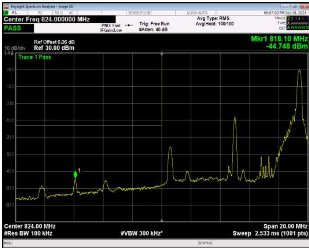
Band5 16QAM BW=10MHz Channel=20450 RB Size=50 Position=#0
