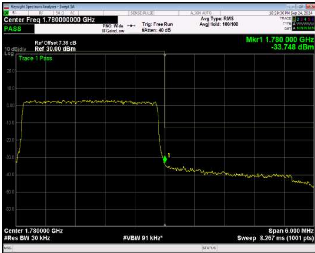
Band66 16QAM BW=3MHz Channel=132657 RB Size=1 Position=#0
