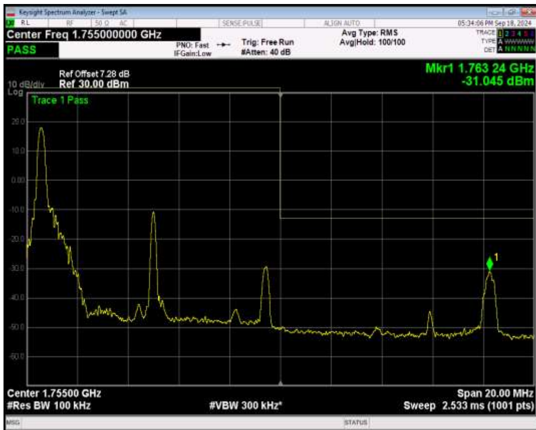
Band4 16QAM BW=10MHz Channel=20350 RB Size=50 Position=#0
