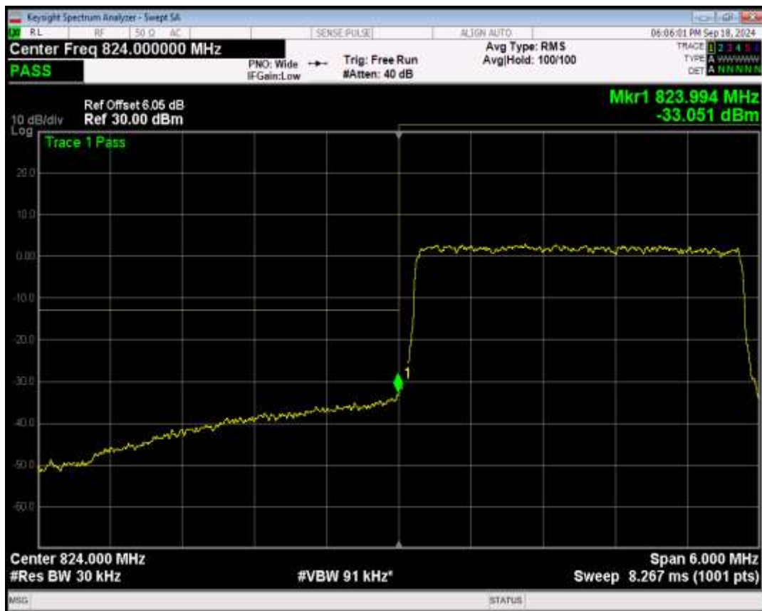
Band5 QPSK BW=3MHz Channel=20635 RB Size=1 Position=#0
