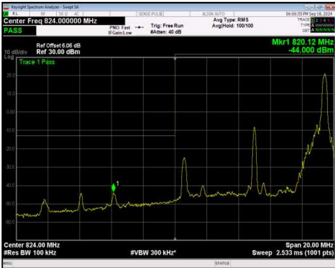
Band5 QPSK BW=10MHz Channel=20450 RB Size=50 Position=#0
