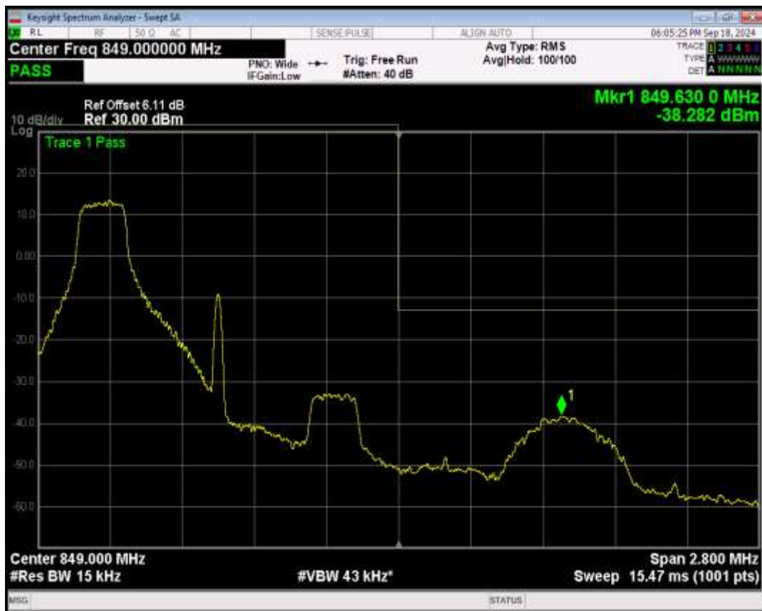
Band5 16QAM BW=1.4MHz Channel=20407 RB Size=6 Position=#0
