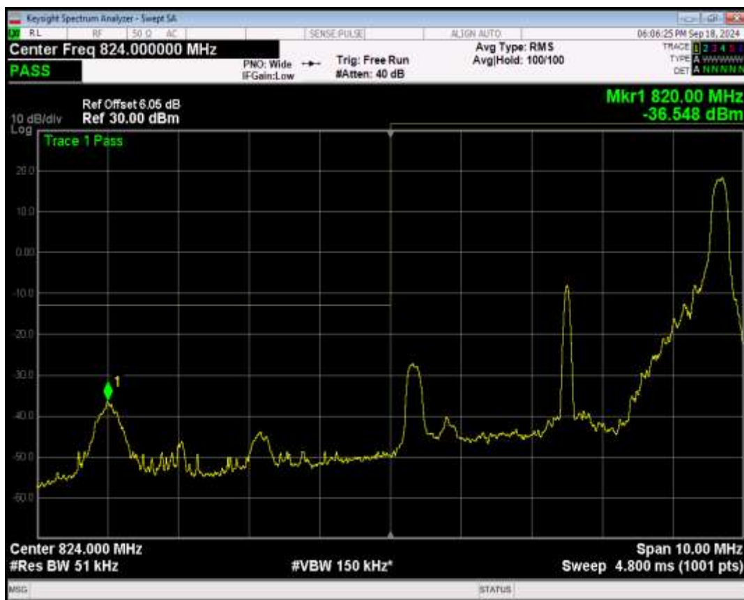
Band5 QPSK BW=5MHz Channel=20425 RB Size=25 Position=#0
