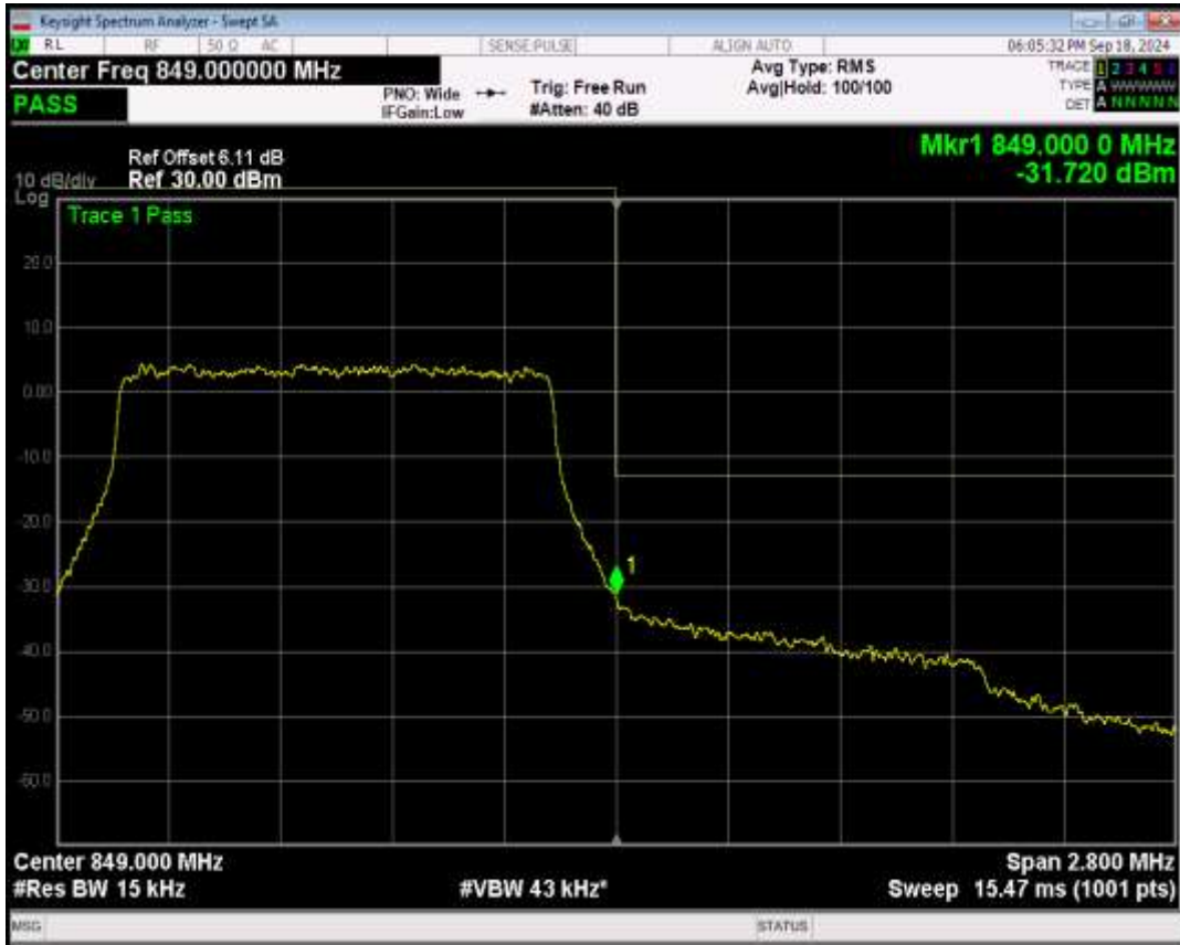
Band5 16QAM BW=1.4MHz Channel=20643 RB Size=1 Position=#0
