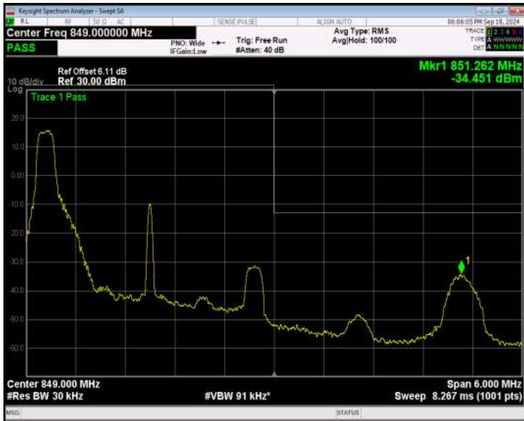
Band5 QPSK BW=3MHz Channel=20635 RB Size=1 Position=#Max
