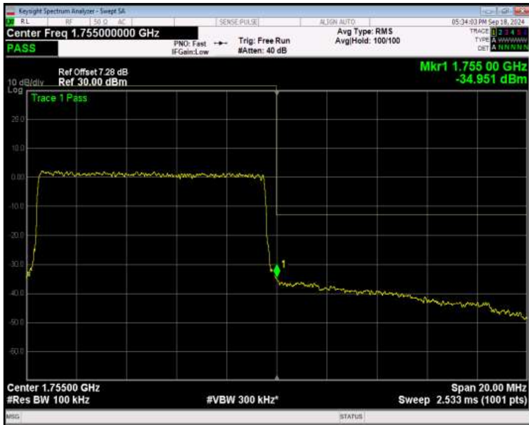
Band4 16QAM BW=10MHz Channel=20350 RB Size=1 Position=#0
