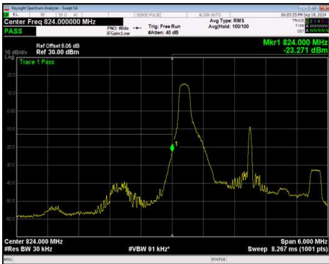
Band5 16QAM BW=3MHz Channel=20415 RB Size=1 Position=#Max
