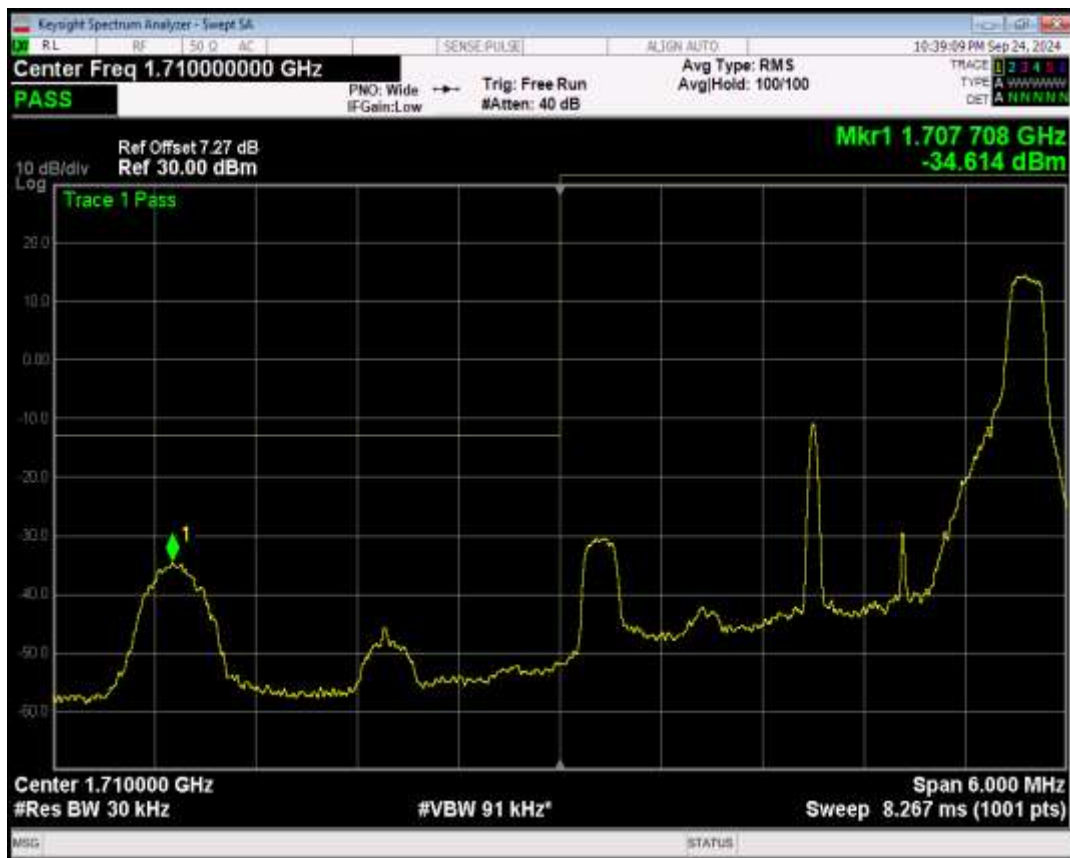
Band66 QPSK BW=3MHz Channel=131987 RB Size=15 Position=#0
