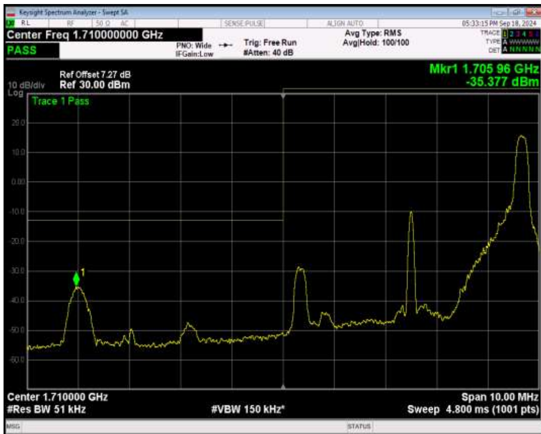
Band4 QPSK BW=5MHz Channel=19975 RB Size=25 Position=#0
