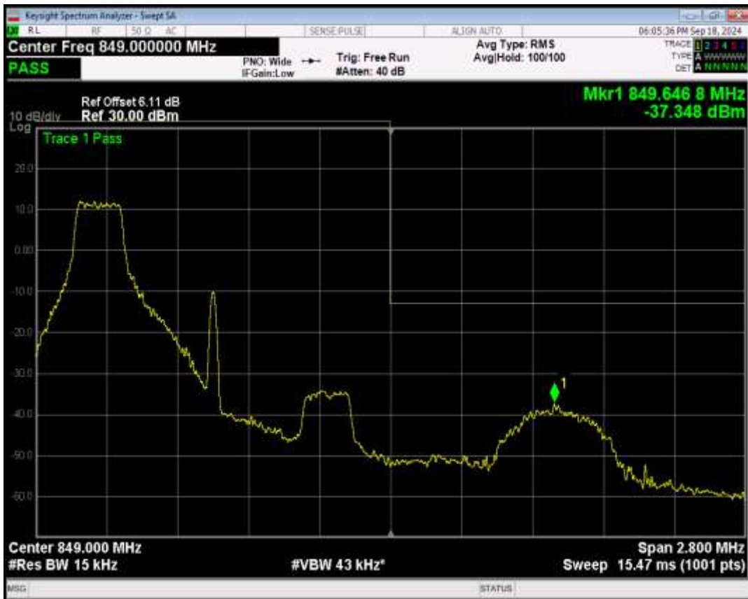
Band5 16QAM BW=1.4MHz Channel=20643 RB Size=1 Position=#Max
