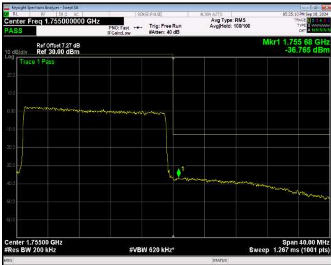
Band41 QPSK BW=5MHz Channel=40115 RB Size=1 Position=#0
