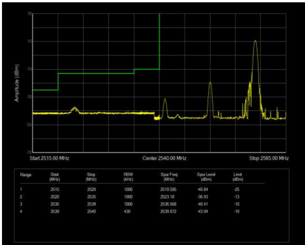
Band41 QPSK BW=20MHz Channel=40190 RB Size=100 Position=#0
