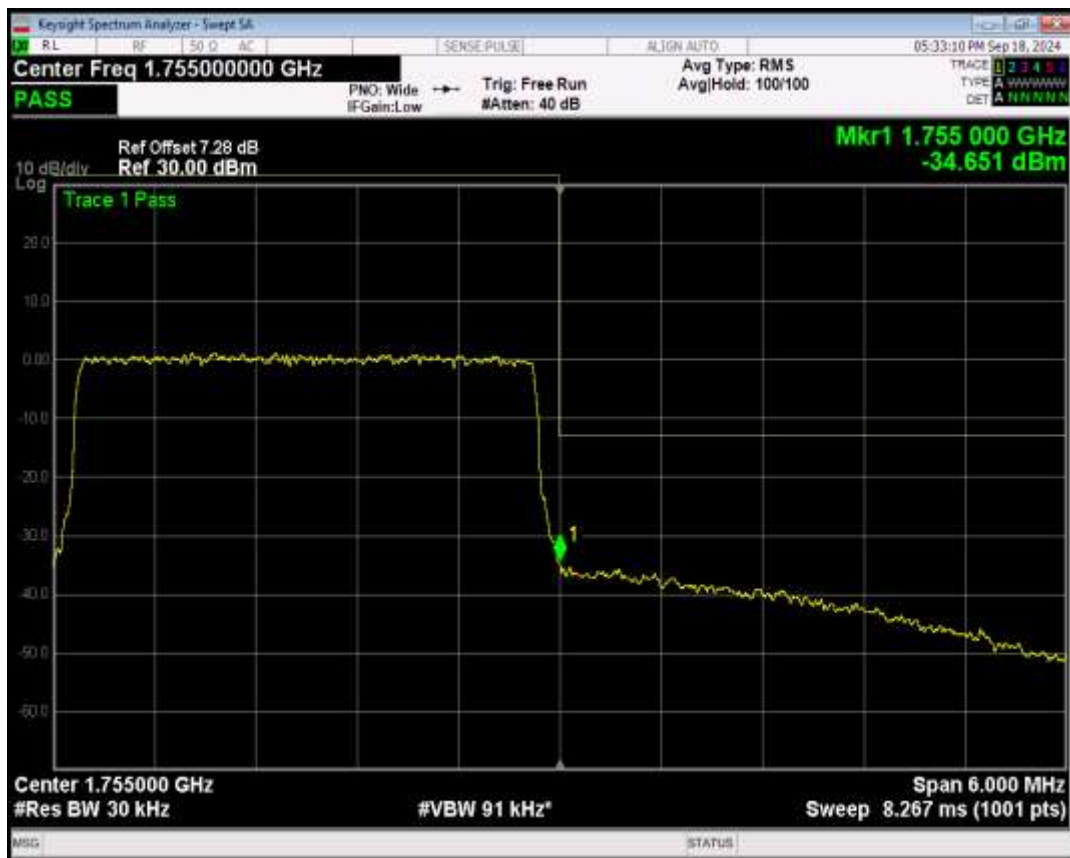
Band4 QPSK BW=5MHz Channel=19975 RB Size=1 Position=#0
