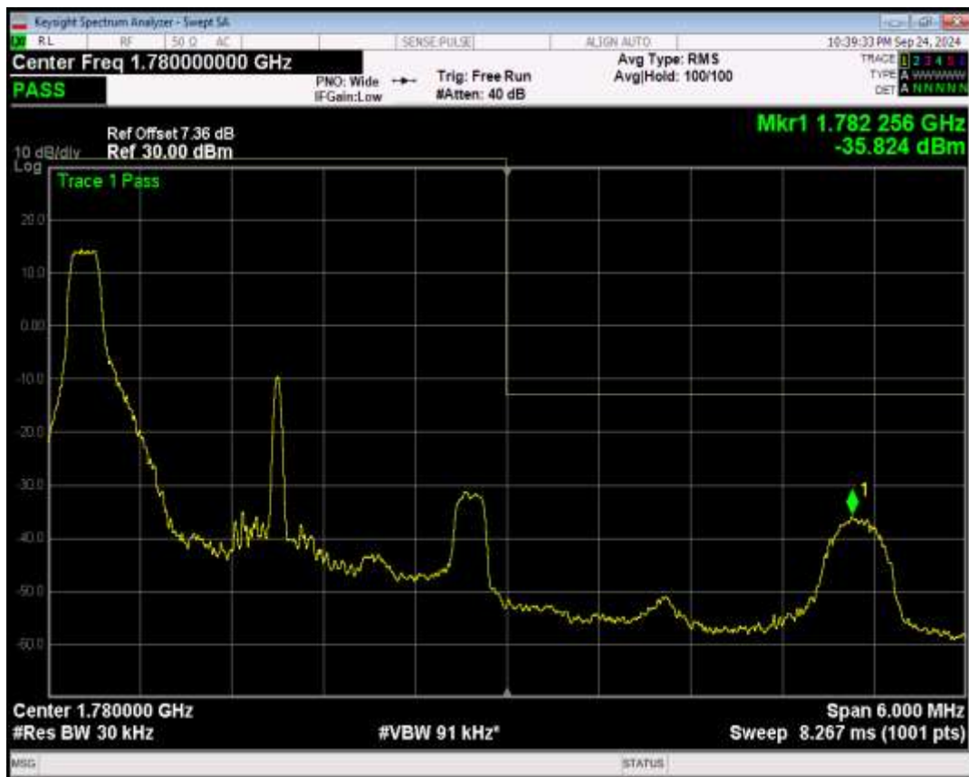
Band66 16QAM BW=3MHz Channel=132657 RB Size=1 Position=#Max
