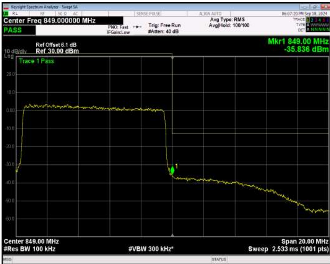
Band66 QPSK BW=3MHz Channel=131987 RB Size=1 Position=#0
