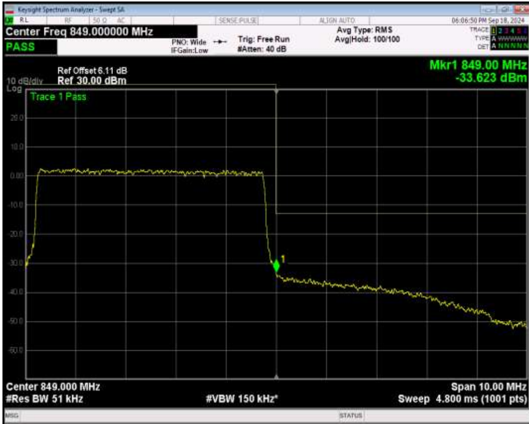
Band5 QPSK BW=10MHz Channel=20450 RB Size=1 Position=#Max
