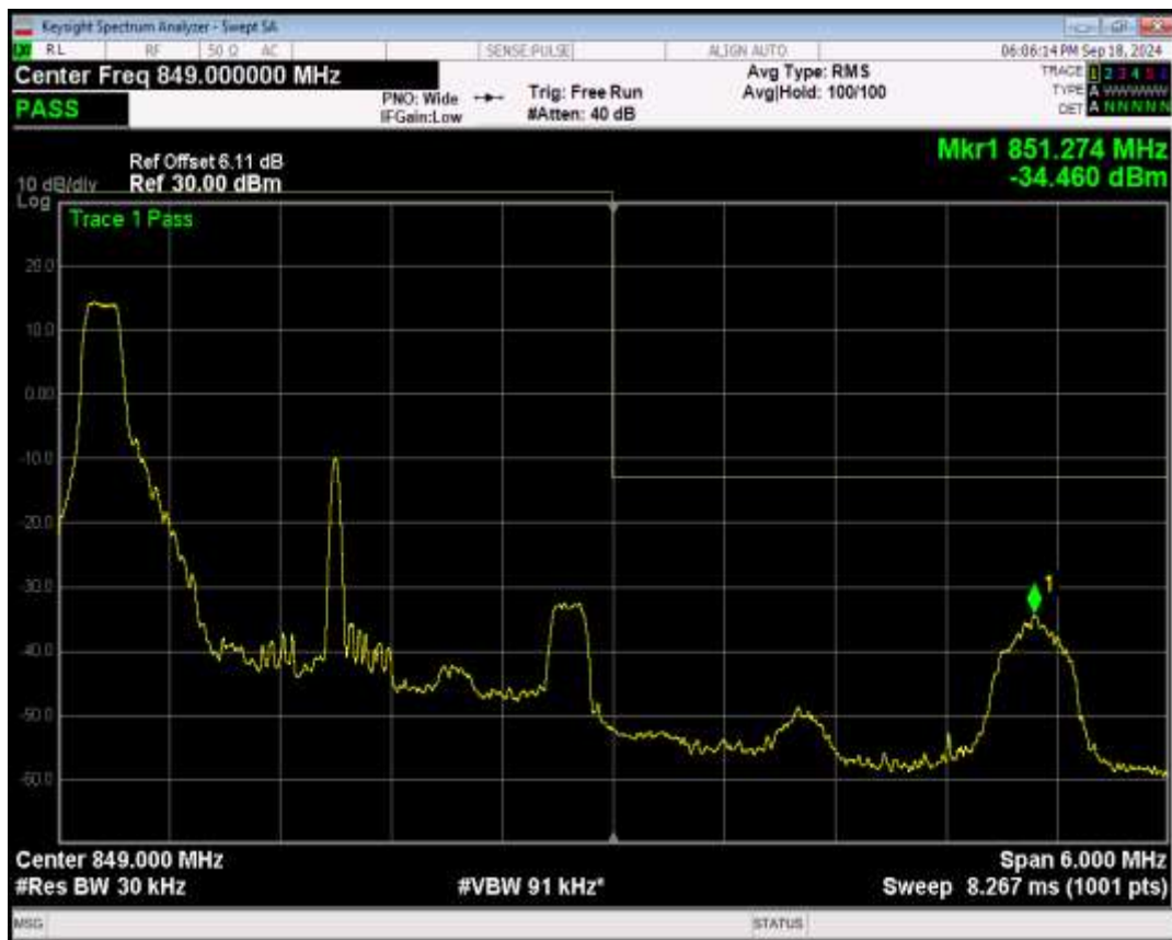
Band5 16QAM BW=3MHz Channel=20635 RB Size=1 Position=#Max
