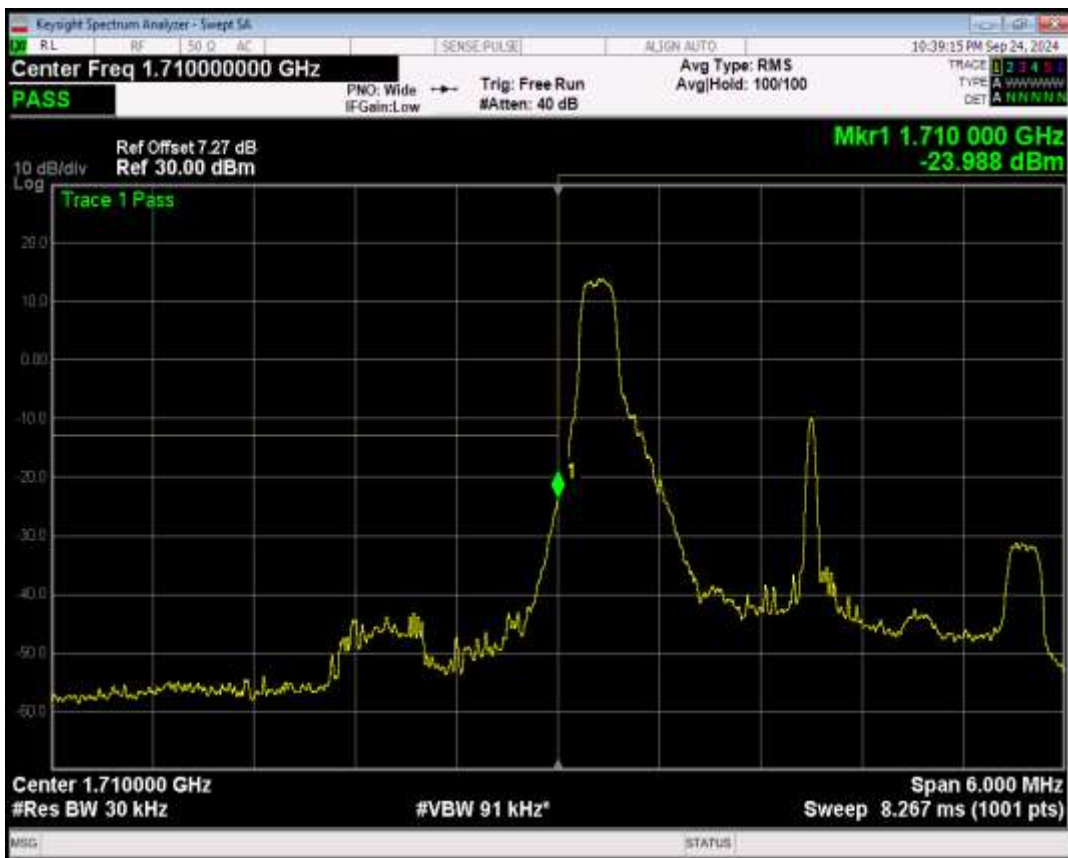
Band66 16QAM BW=3MHz Channel=131987 RB Size=1 Position=#Max
