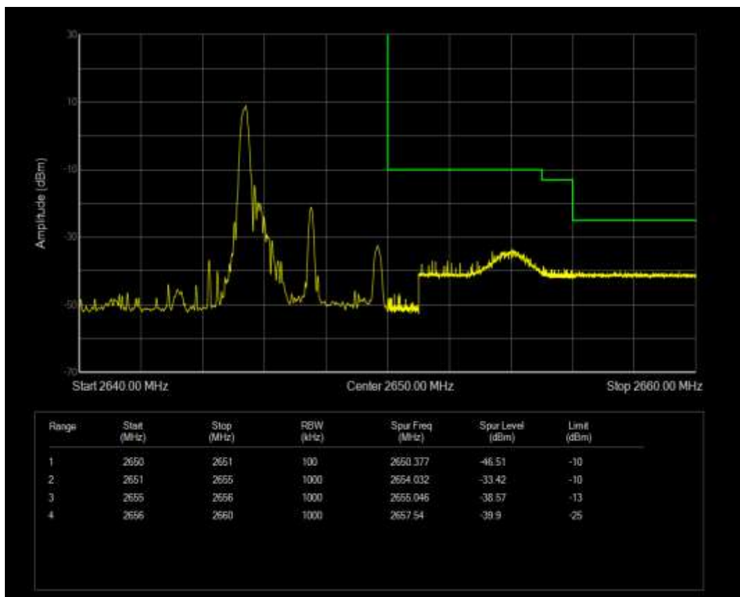
Band41 QPSK BW=5MHz Channel=41165 RB Size=1 Position=#Max
