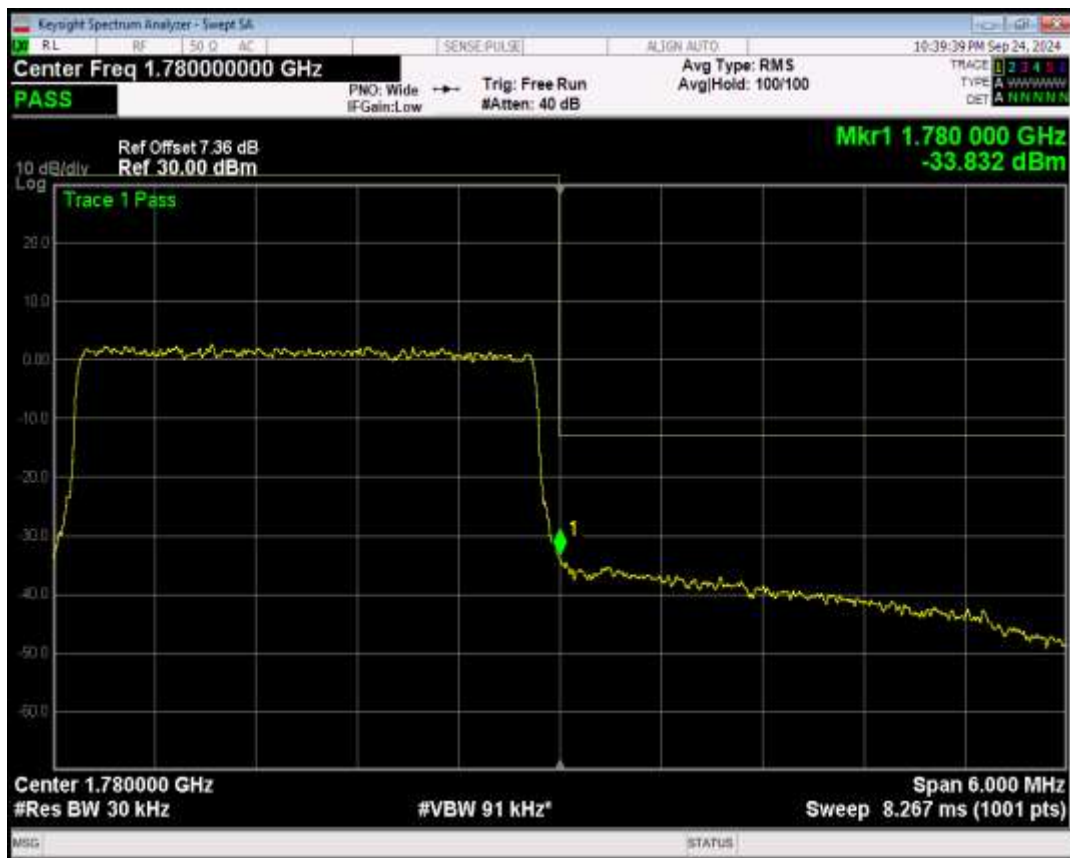
Band7 QPSK BW=5MHz Channel=20775 RB Size=1 Position=#0
