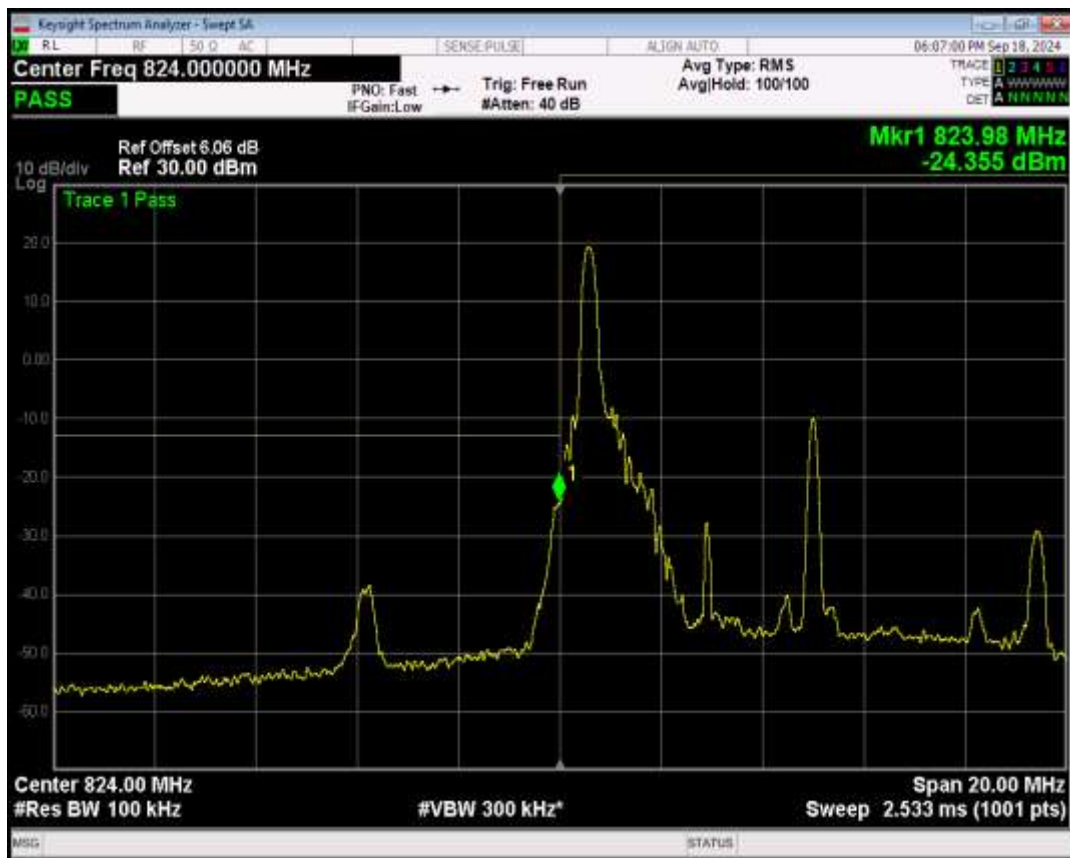
Band5 16QAM BW=10MHz Channel=20450 RB Size=1 Position=#Max
