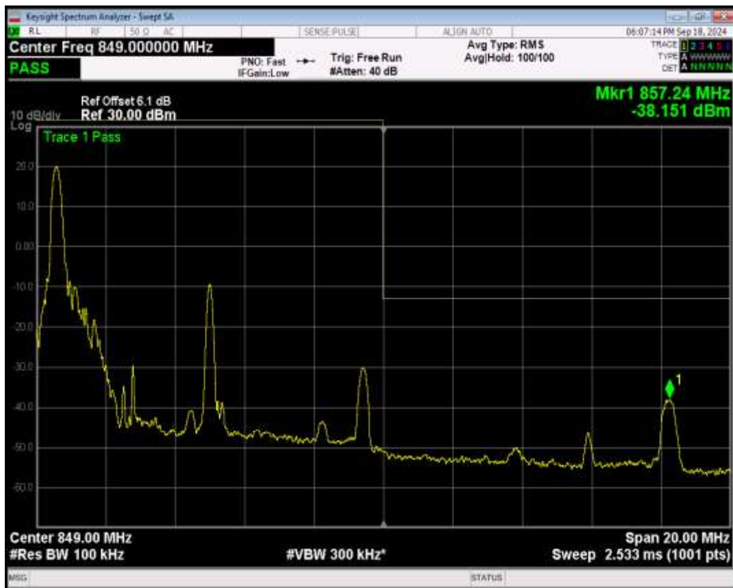
Band5 16QAM BW=10MHz Channel=20600 RB Size=1 Position=#Max
