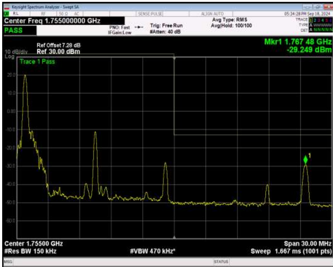
Band4 QPSK BW=15MHz Channel=20325 RB Size=1 Position=#Max
