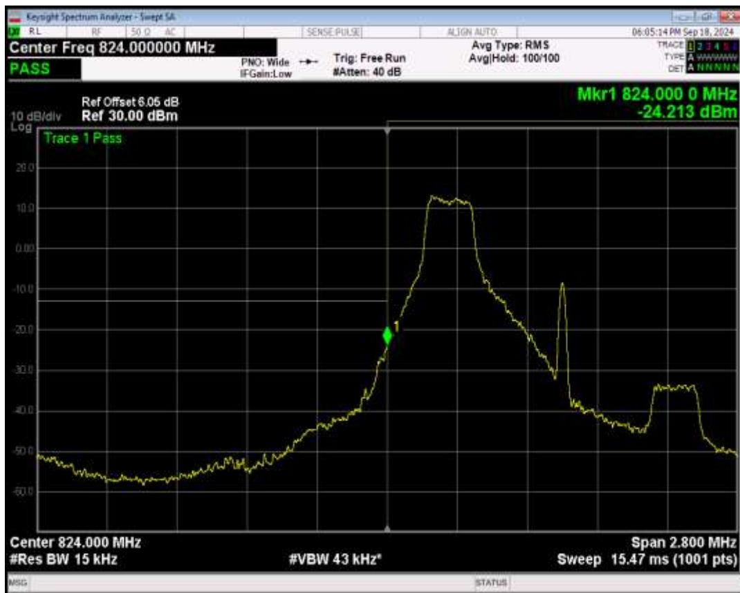
Band5 16QAM BW=1.4MHz Channel=20407 RB Size=1 Position=#Max
