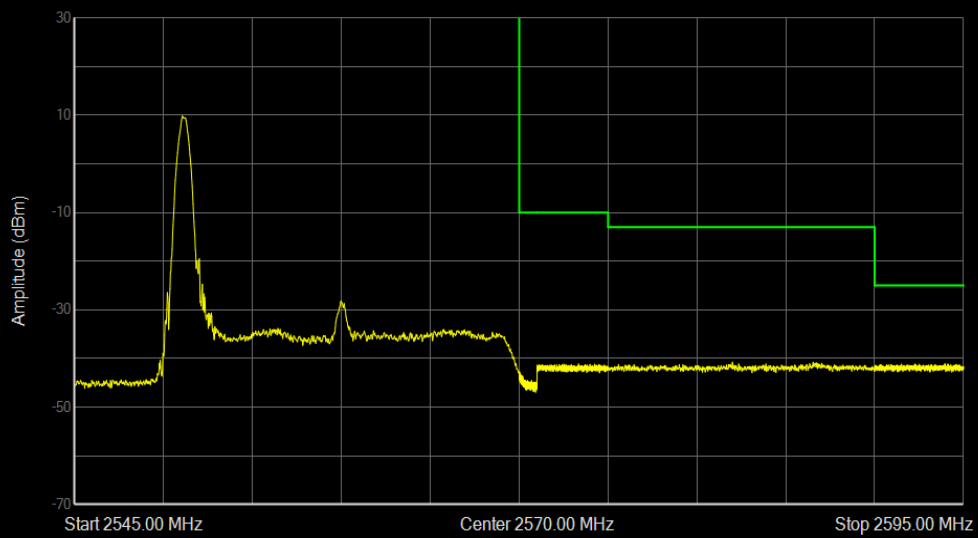
Band7 QPSK BW=20MHz Channel=21350 RB Size=1 Position=#0
