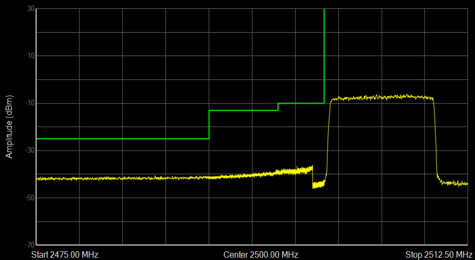
Band7 QPSK BW=10MHz Channel=20800 RB Size=50 Position=#0
