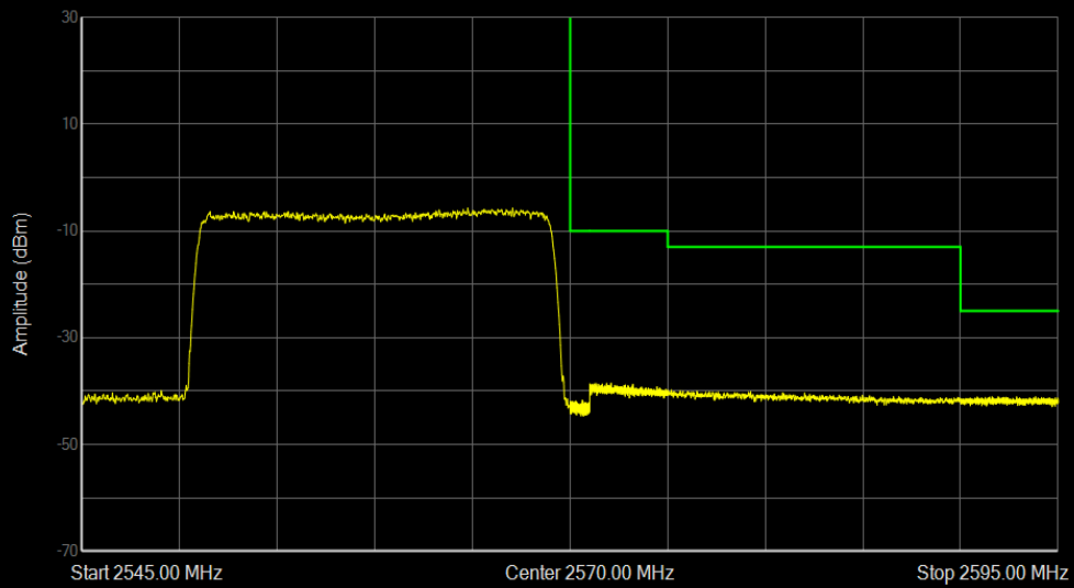
Band7 QPSK BW=20MHz Channel=21350 RB Size=100 Position=#0
