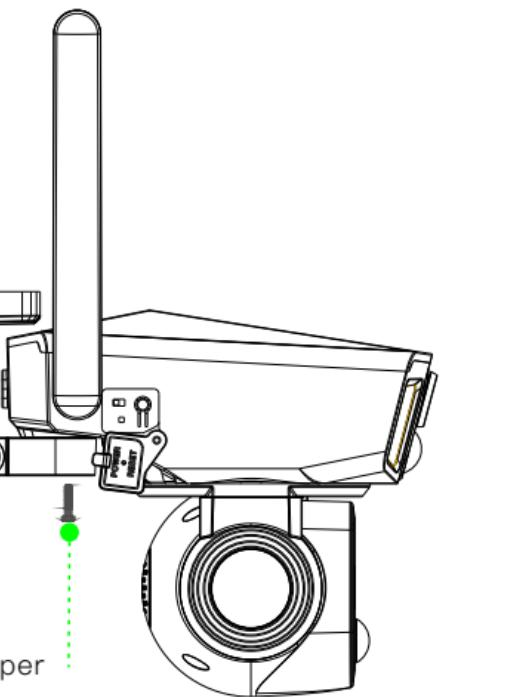
After adjusting the tilt angle of the wide-angle camera, tighten the thumbscrew to fix the lens position.
