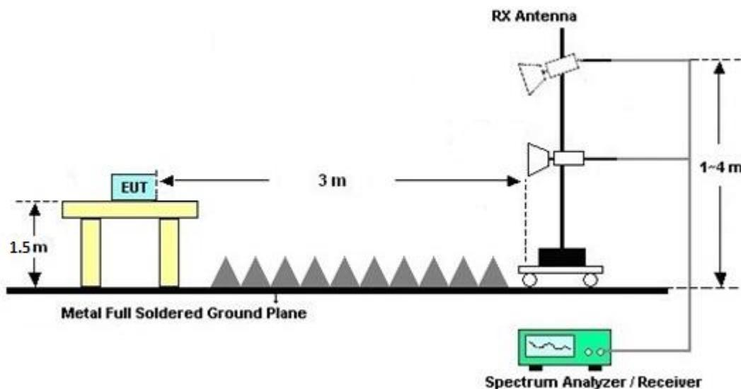
For radiated test above 18GHz
