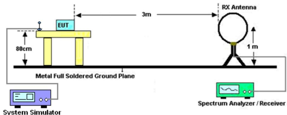
For radiated test from 30MHz to 1GHz
