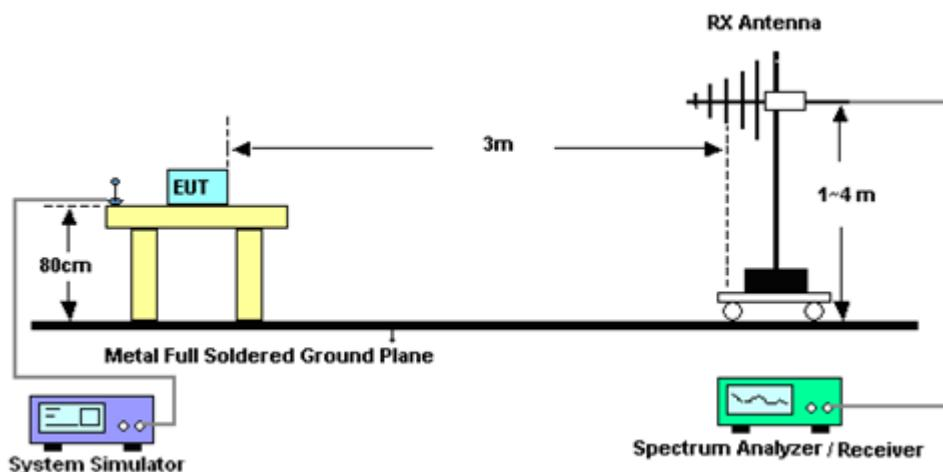
For radiated test from 1GHz to 18GHz
