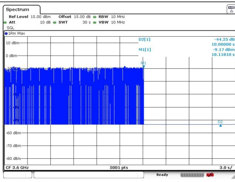
[Step 5] Setup with 3670-3690MHz & power level 17dBm/MHz
