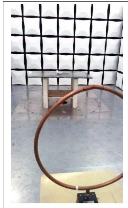
**Radiated Spurious Emissions: 30 MHz to 1000 MHz**
