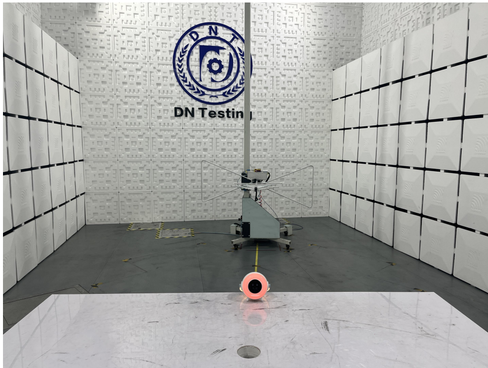
Radiated Emission Test View (Below 1G)
