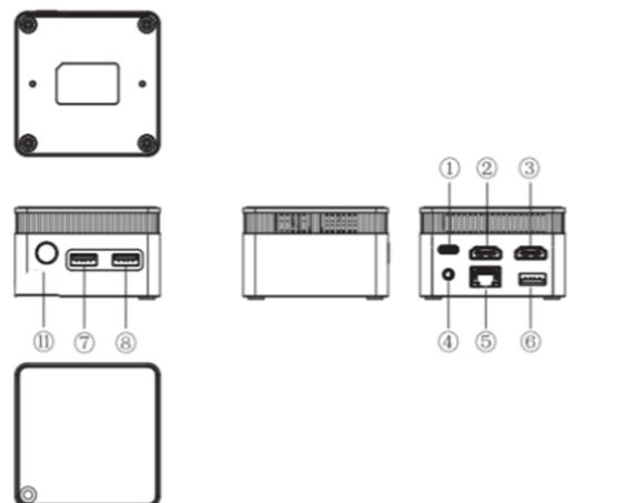
1, Power Input 2,HD Port 3,HD Port 4, Earphone 5, RJ45
