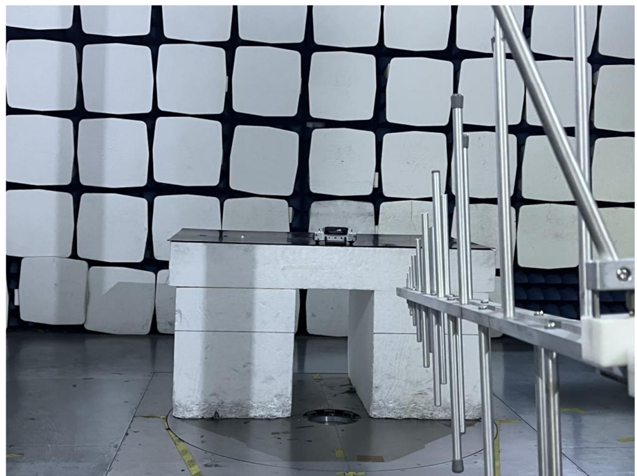
Radiation Emission Test Setup (30MHz to 1GHz)
