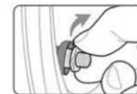
③Rotate to the tyre valve according to the position marking on the sensor nut
