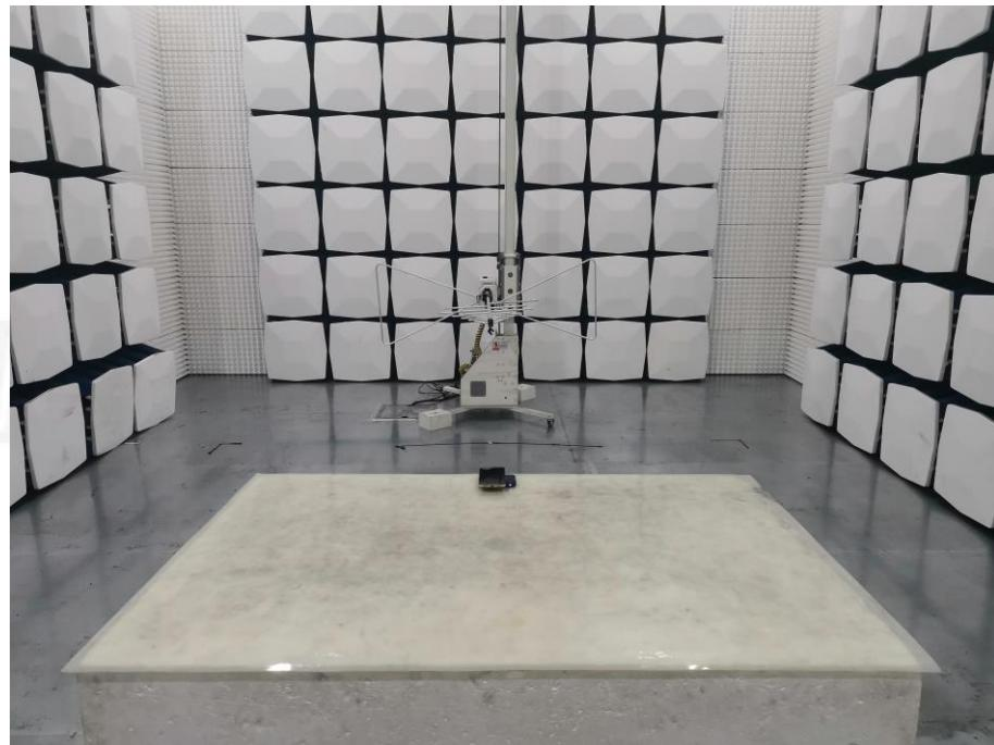
Radiated band emission (9KHz-30MHz):
