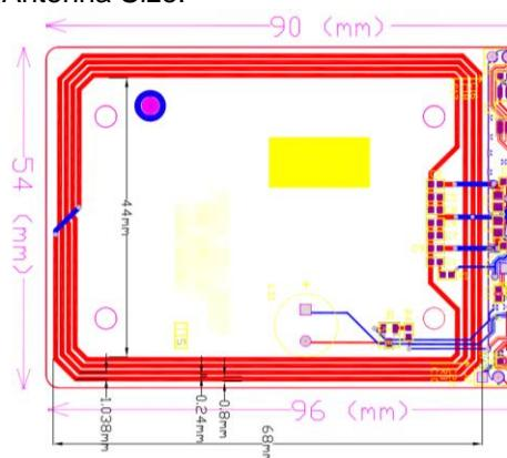
The mounting of the antenna is fixed to the radio module and no other antenna should be used.
