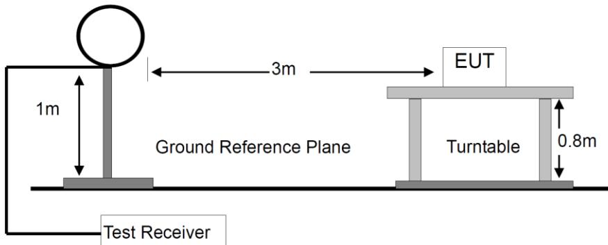
For Radiated Emission 30-1000MHz
