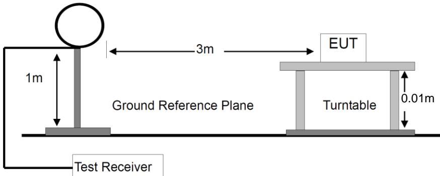
For Radiated Emission 30-1000MHz
