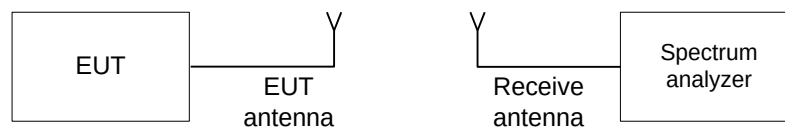
Figure 7.7.1 Band edge emission test setup
