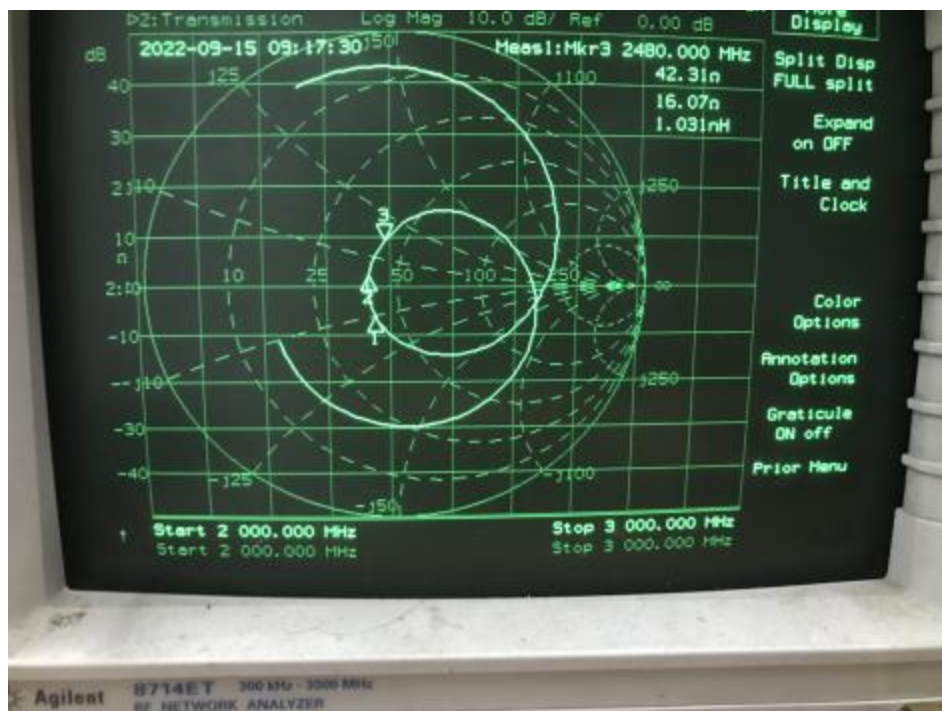
Figure 3 keyboard Antenna S11
