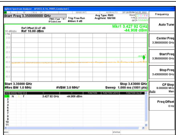
5G NR n77 20MHz QPSK Low channel second segment
