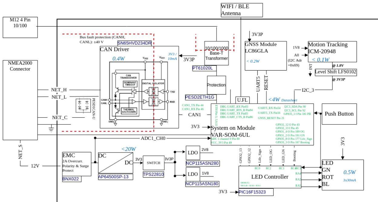
The Orca Core's internal design includes the following key components:
