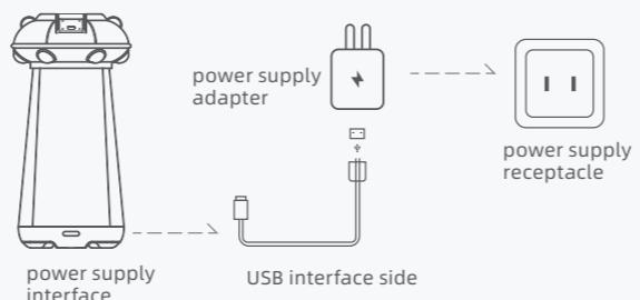
Connect the power cord to the power adapter, and then connect to the product's power connector. The power adapter is plugged into a power outlet and the connection is successful.
