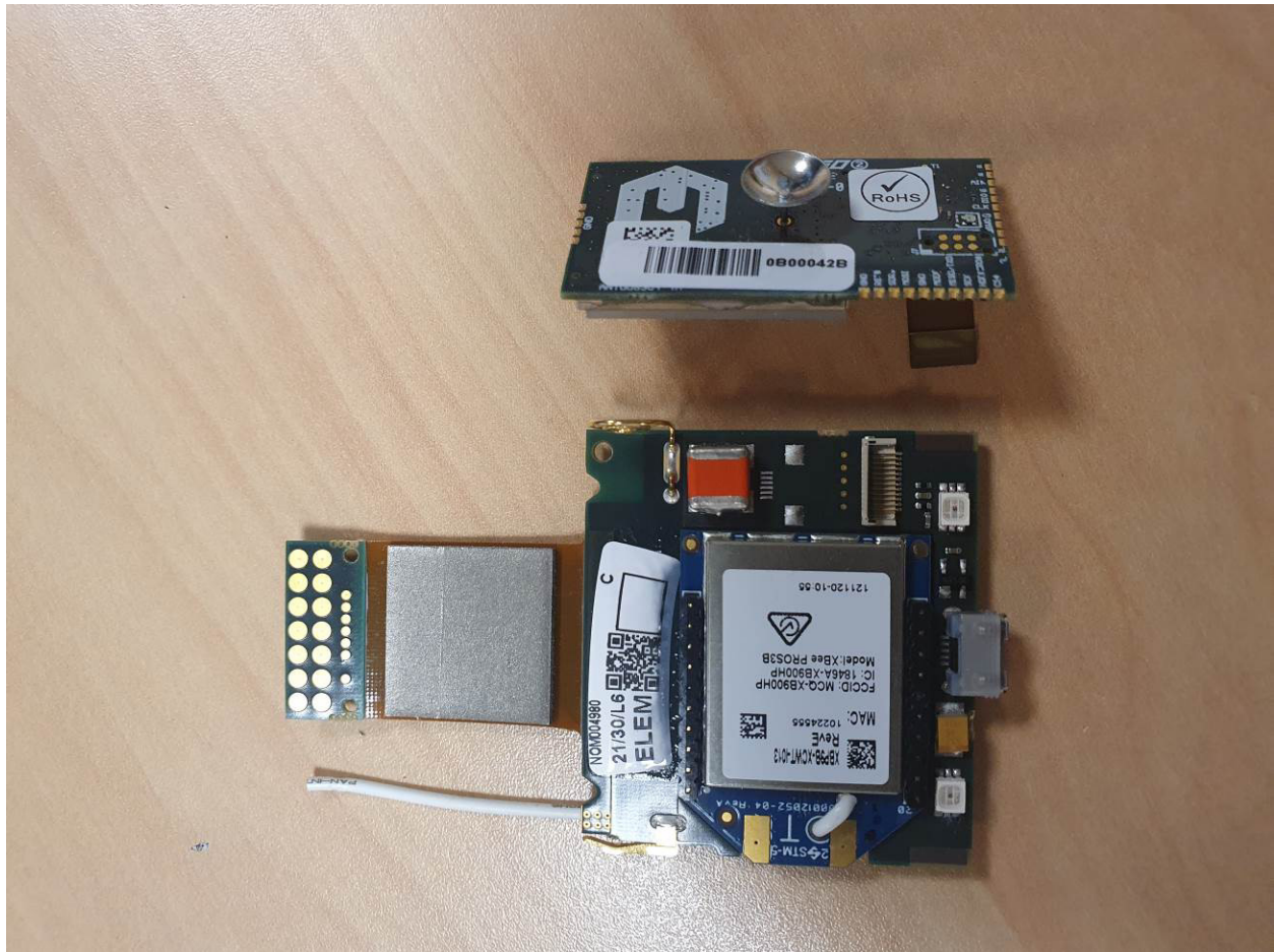
Figure 10. PCBA removed from plastic housing, Top View, accessory board removed.
