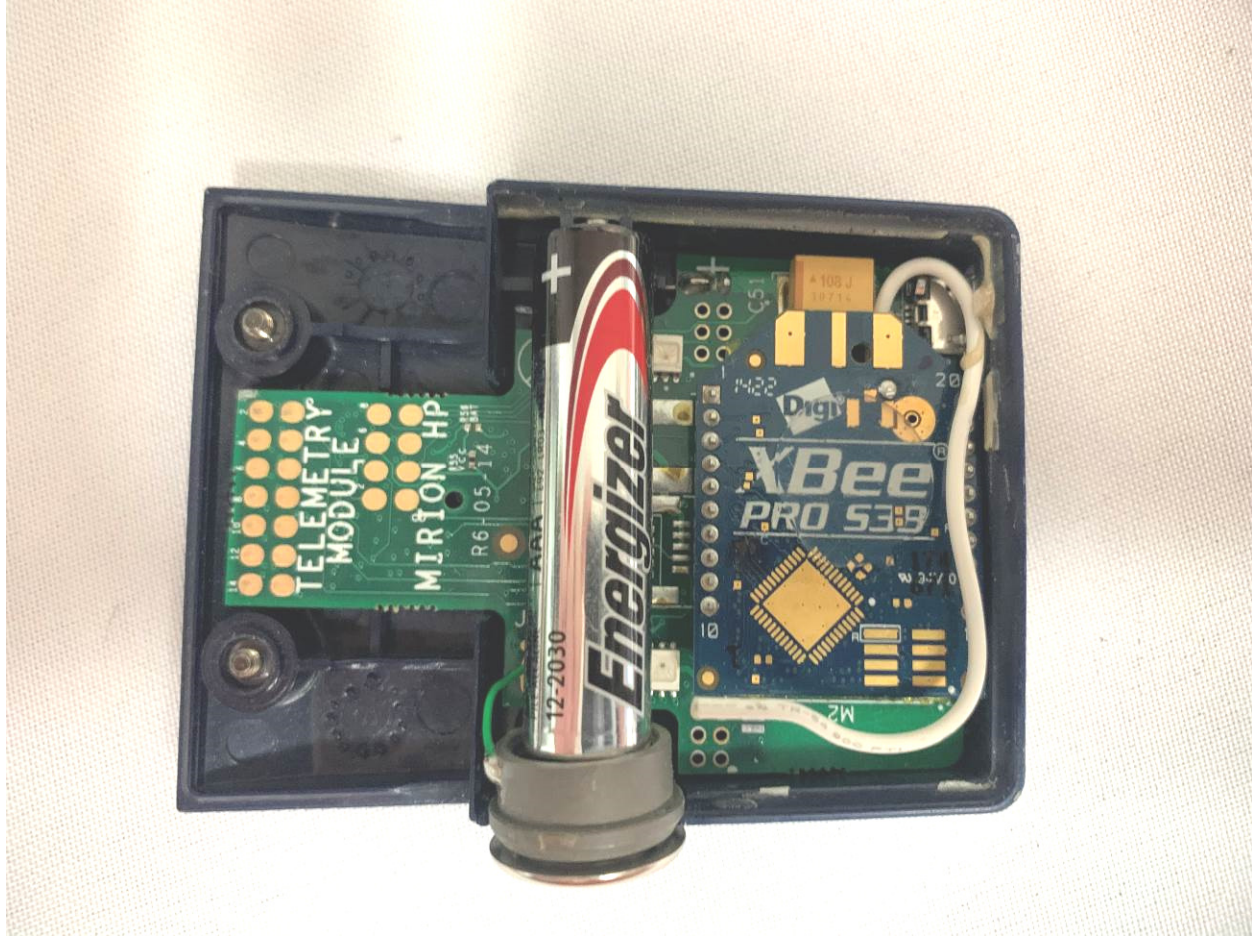
Figure 5. Transmitter Section, Top cover removed
