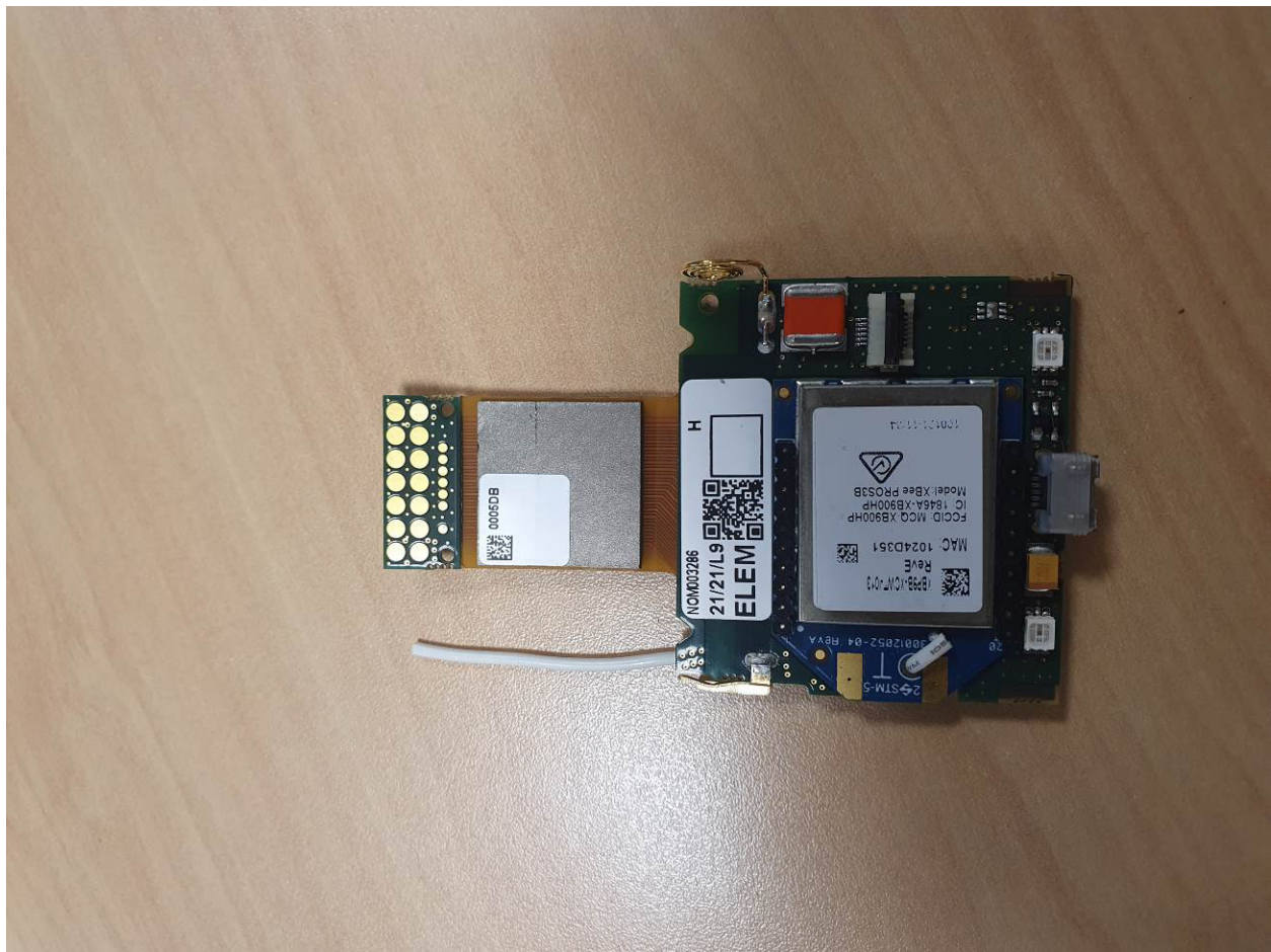
Figure 12. PCBA removed from plastic housing, Top View
