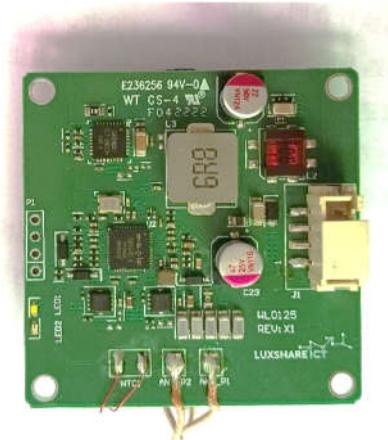
This specification defines the electrical, reliability, EMC and REL requirements of the wireless charging transmitter base. The wireless charging system is based on electromagnetic induction technology.
