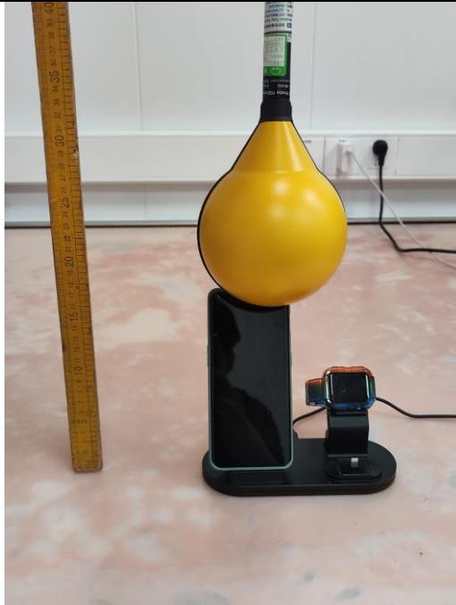
**H-Field Strength-15cm****Test Position - Exposure photo from side edge surface-Left**
