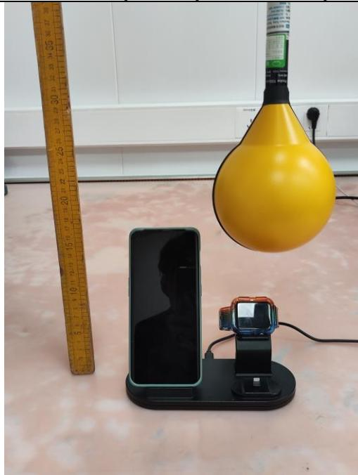
**H-Field Strength-15cm****Test Position - Exposure photo from side edge surface-Left**
