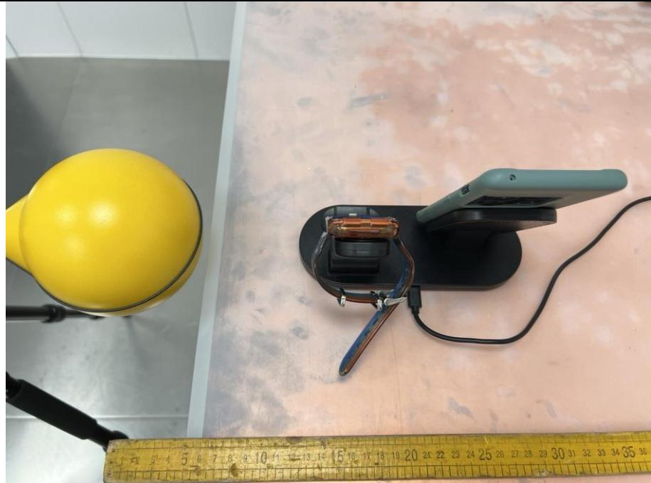
**H-Field Strength- 15 cm****Test Position - Exposure photo from top surface**
