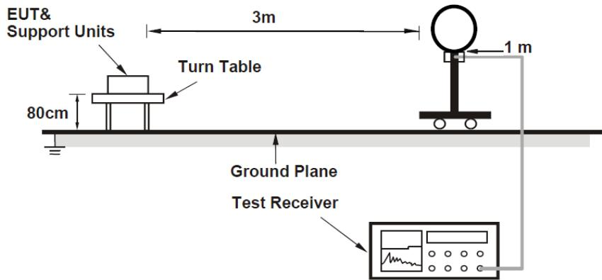
For Radiated emission 30MHz to 1GHz
