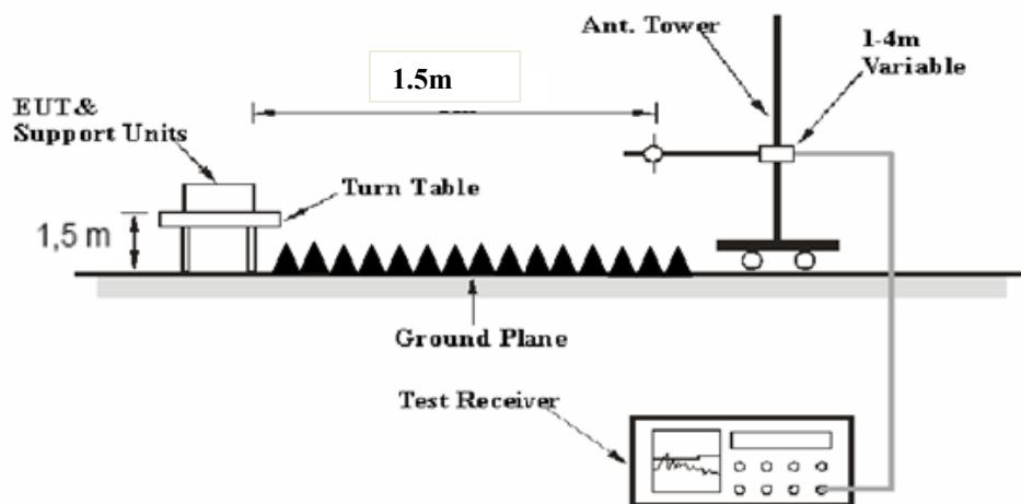
The radiated emission were performed in the 3 meters chamber test site, using the setup accordance with the ANSI C63.4-2014. The specification used was with the FCC Part 15 B Class B limits.
