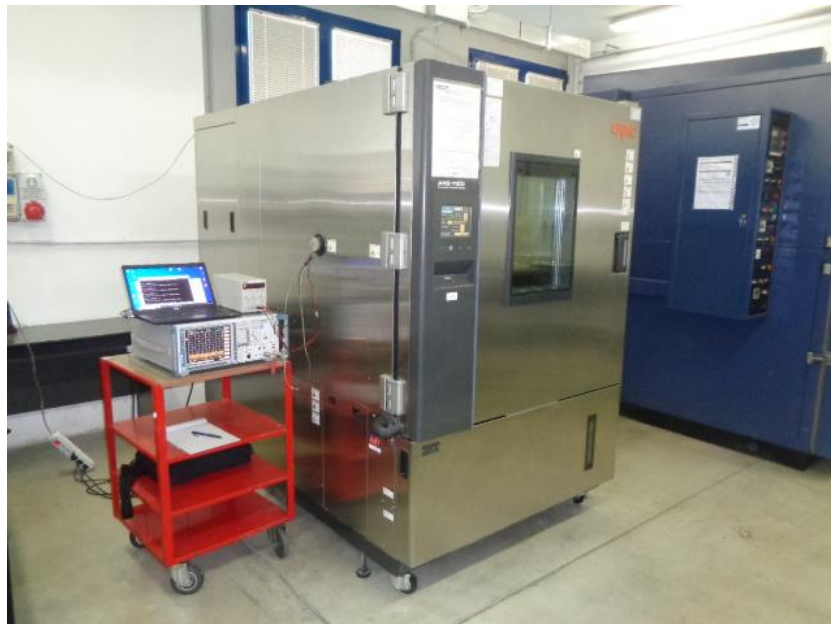
Figure 9.1-2: Antenna port testing set-up in climatic chamber
