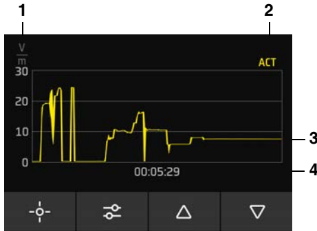
Fig. 10: Graphic display in the TIMER LOGGING operating mode after calling it up in the DATA LOGGER
