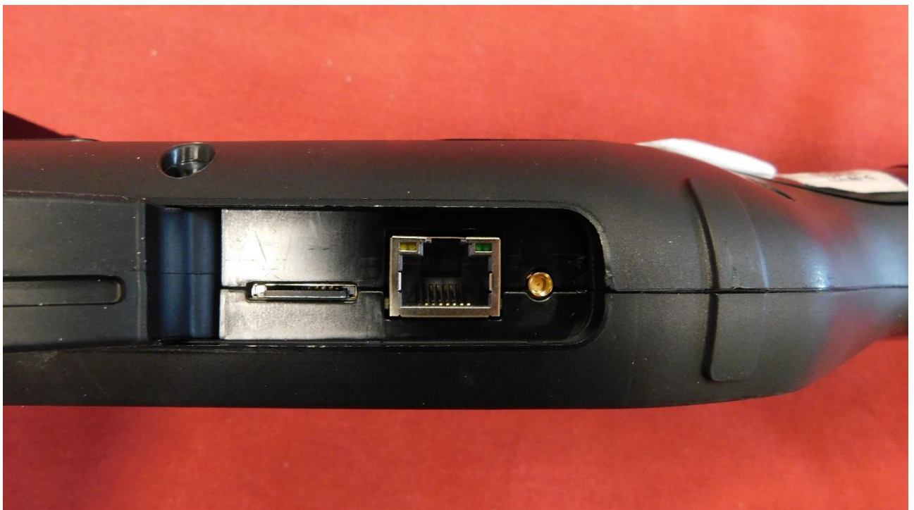
Picture 8: EUT – Ethernet port
