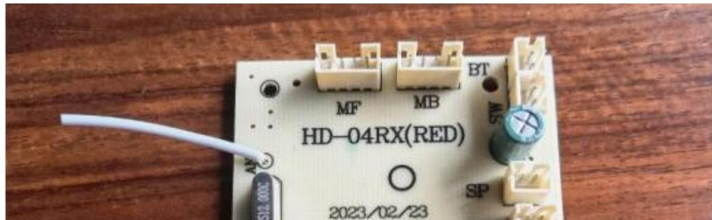
Note: 2.4G antenna specification is 7 core 0.14 copper diameter bare copper wire outer wire diameter 1.3MM wire, white, length of 35MM, wire head peeling 3MM tin. Meet the environmental protection standards: EU EN 71 (19E), ROHS, PAHS, 6P ~ 16P, Europe and America CPSIA , HR 4040.
