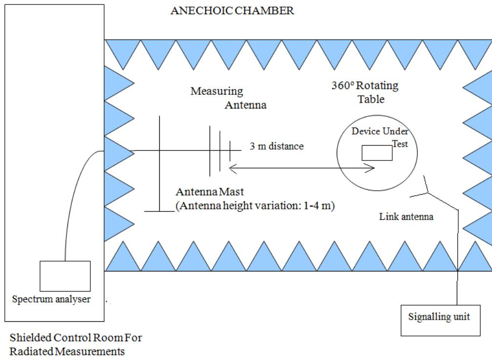
Radiated measurements above 1 GHz:
