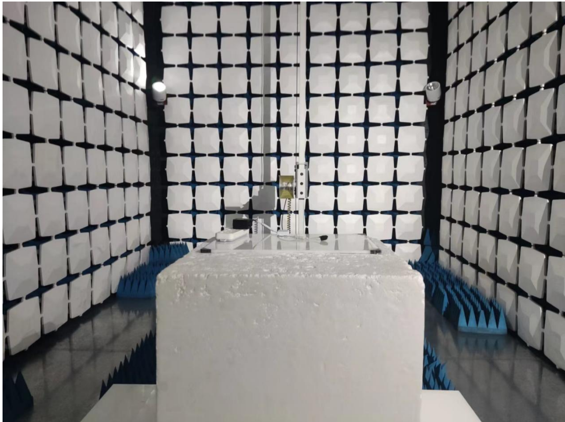
Above 1GHz for radiated emission test setup
