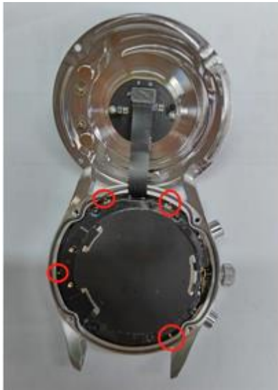
Metal middle frame as the antenna funtion
