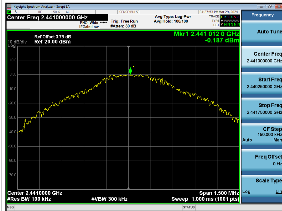
Tx. Spurious NVNT 1-DH5 2441MHz Ant1 Emission
