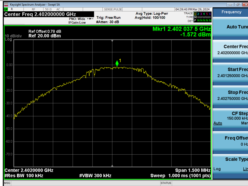
Tx. Spurious NVNT 1-DH5 2402MHz Ant1 Emission
