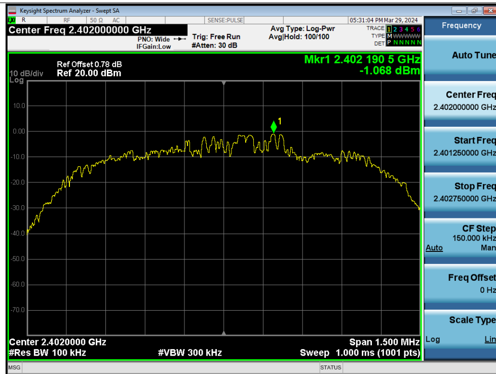
Tx. Spurious NVNT 3-DH5 2402MHz Ant1 Emission
