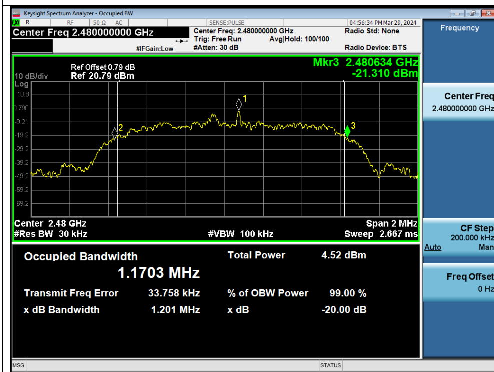
-20dB Bandwidth NVNT 2-DH5 2480MHz Ant1
