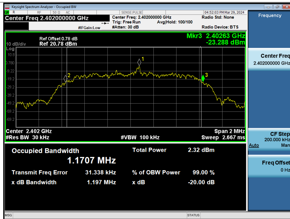
-20dB Bandwidth NVNT 2-DH5 2402MHz Ant1
