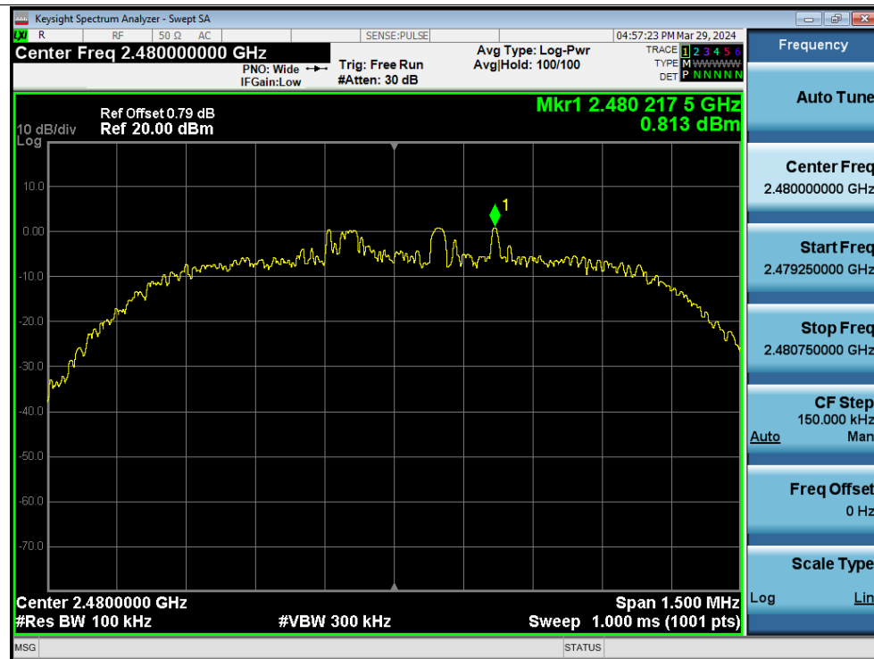
Tx. Spurious NVNT 2-DH5 2480MHz Ant1 Emission
