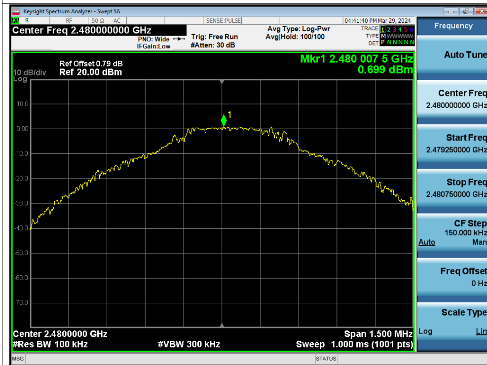
Tx. Spurious NVNT 1-DH5 2480MHz Ant1 Emission
