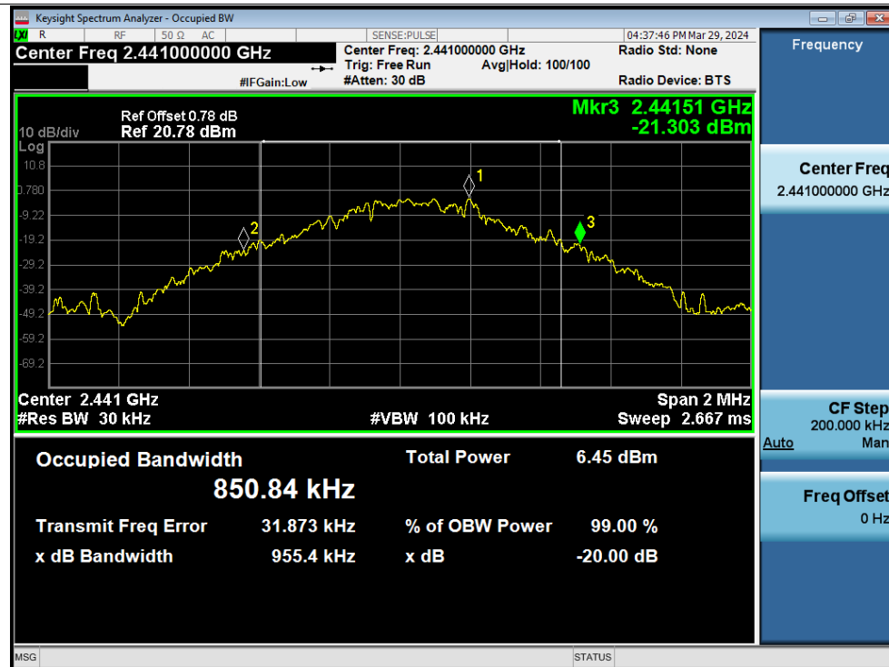
-20dB Bandwidth NVNT 1-DH5 2441MHz Ant1
