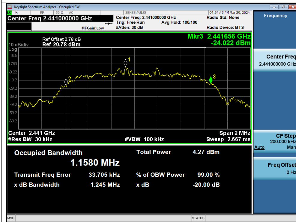
-20dB Bandwidth NVNT 2-DH5 2480MHz Ant1
