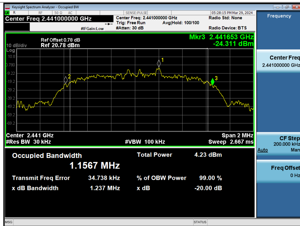
-20dB Bandwidth NVNT 3-DH5 2441MHz Ant1
