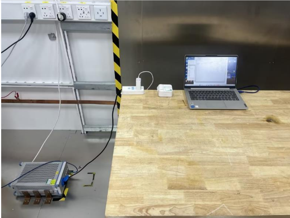
AC Power Line Conducted Emission
