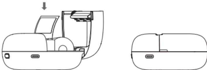
⚠ Only one side of the printing paper can be printed. Please place the printing paper in the correct direction.
