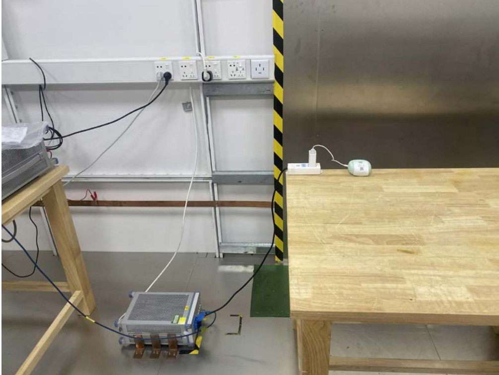
AC Power Line Conducted Emission
