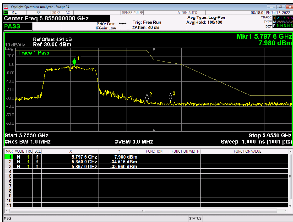
Band Edge NVNT ac80 5775MHz High Ant1
