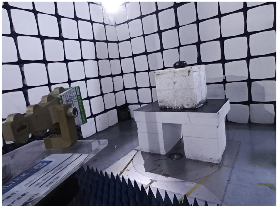
Radiation Emission Test Setup (Above 18GHz)
