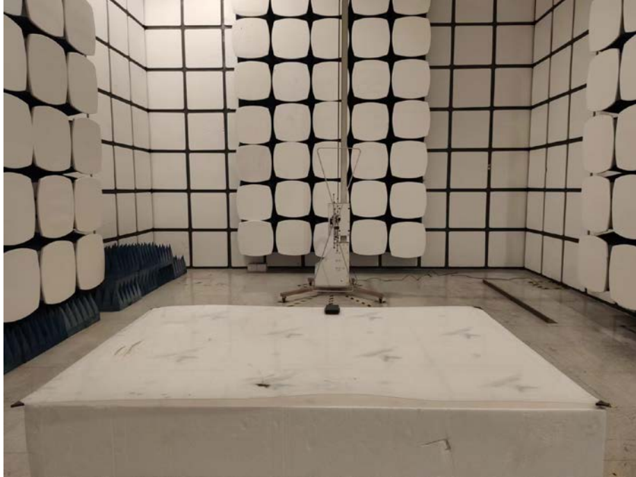
Spurious Emission Test Setup (Below 1GHz)
