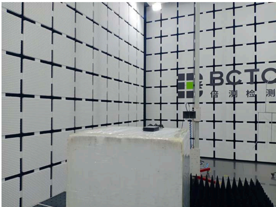
Spurious Emission Test Setup (Above 1GHz)
